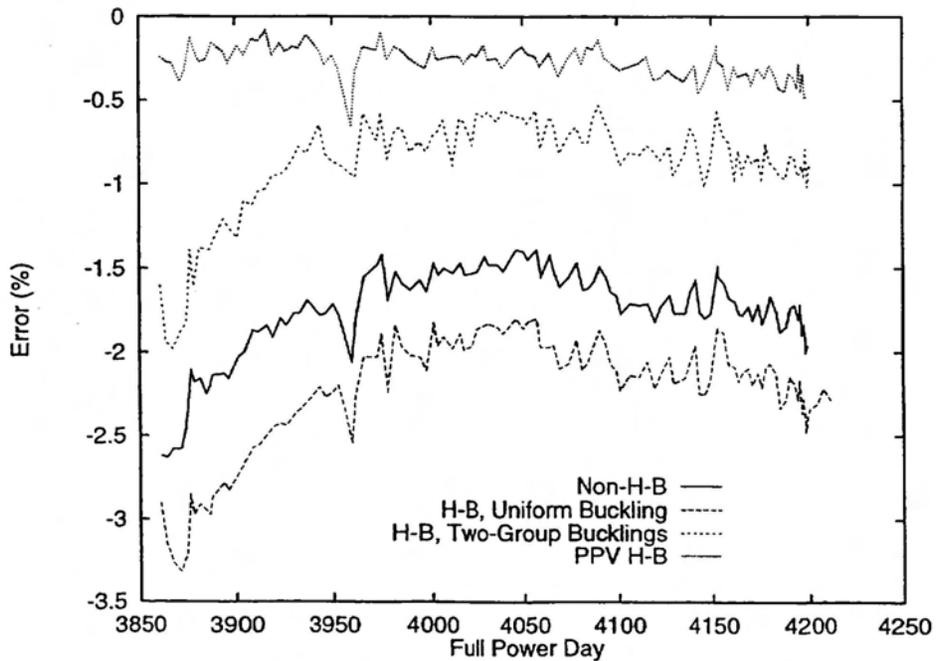
Figure 3: Inner-Core Flux Deviation Variation between RFSP Calculated and Measured Vanadium Detector Readings with Full-Power-Day in PLGS Simulations
