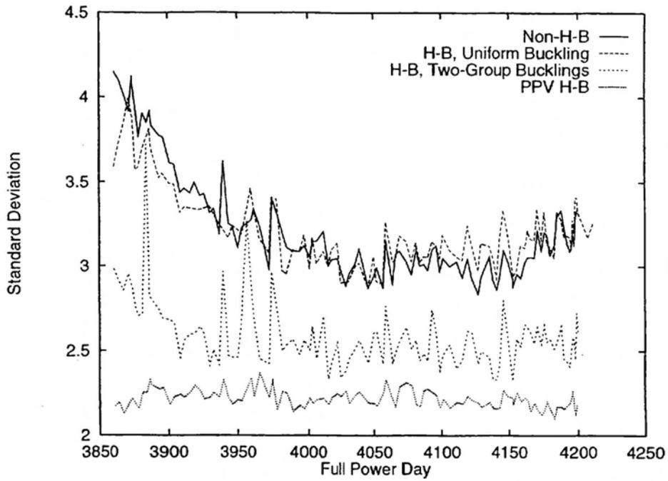
Figure 2: Standard Deviation Variation between RFSP Calculated and Measured Vanadium Detector Readings with Full-Power-Day in PLGS Simulations
