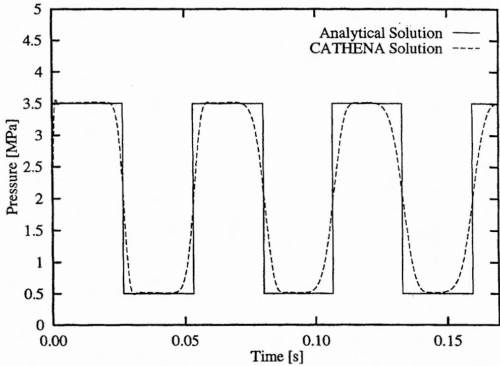
FIGURE 1: Water Hammer Created by an Instantaneous Valve Closure
