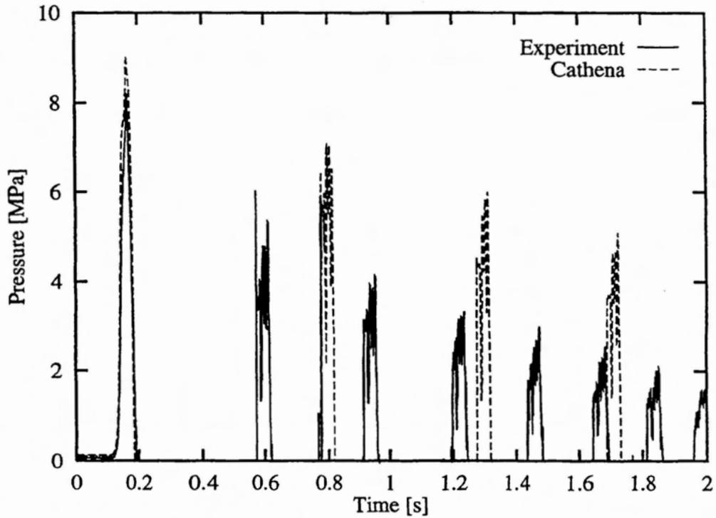
FIGURE 4: Seven Sisters Valve Slam Water Hammer (Large Void Generated) and Corresponding CATHENA Simulation
