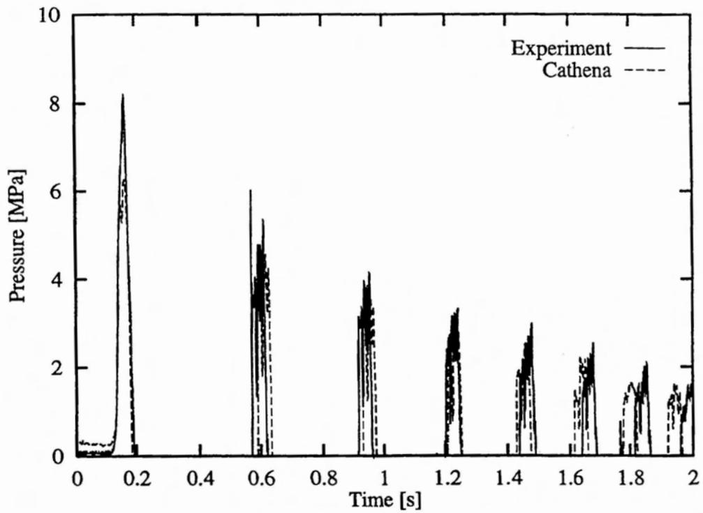
FIGURE 5: Seven Sisters Valve Slam Water Hammer (Large Void Generated) and Corresponding CATHENA Simulation with Adjusted Velocity-dependent Hydraulic Resistance
