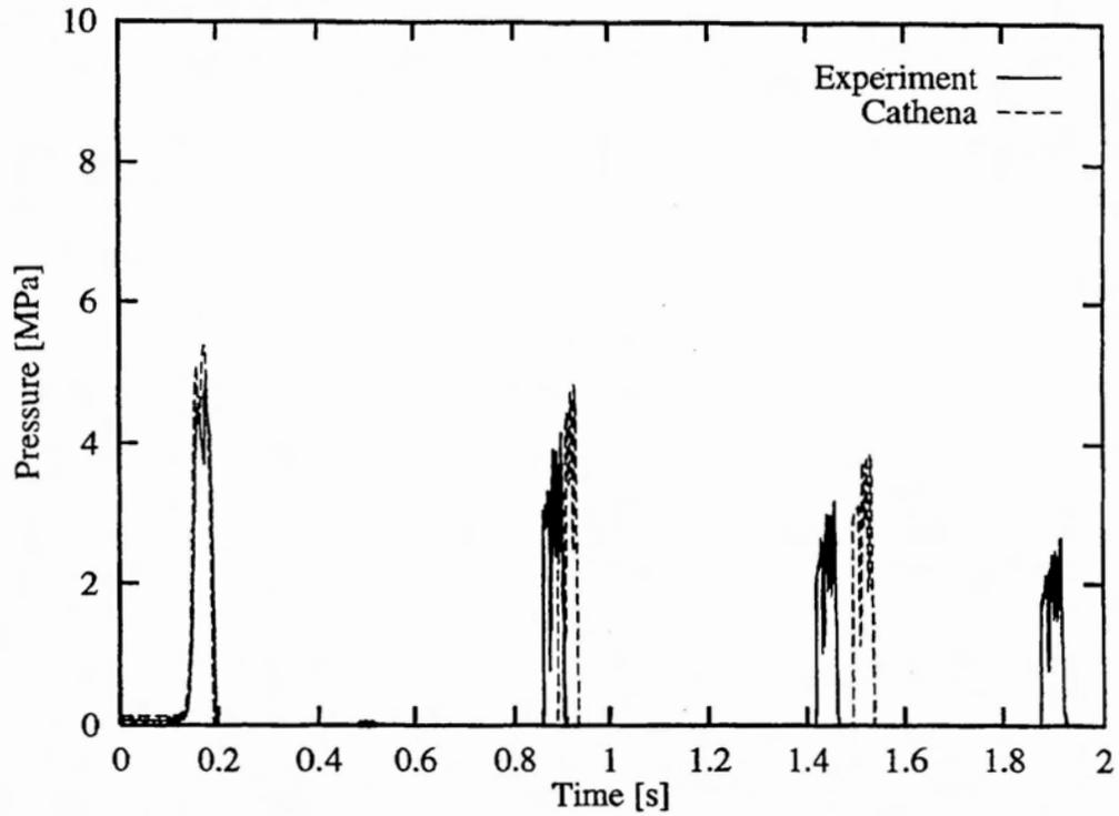
FIGURE 3: Seven Sisters Valve Slam Water Hammer (Small Void Generated) and Corresponding CATHENA Simulation
