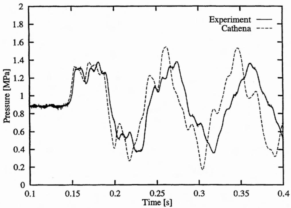
FIGURE 2: Seven Sisters Single Phase Valve Slam Water Hammer and Corresponding CATHENA simulation
