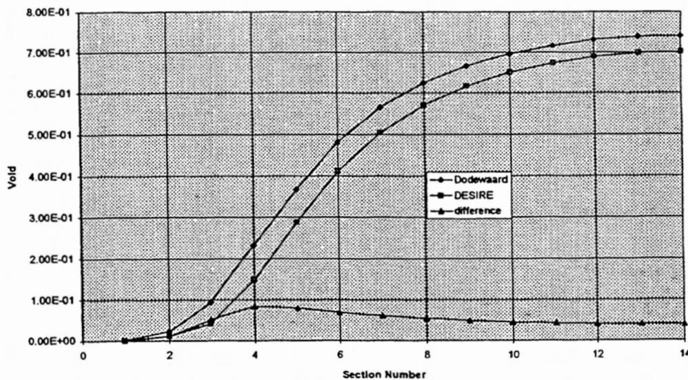
to the figure, it can be seen that the actual DESIRE facility under-estimates the void fraction, relative to the Dodewaard values, at each axial section due to the discrepancy in the rod pitch to diameter ratio. It would appear that this effect represents a constant bias after the fourth axial segment. Thus, it may be possible to correct the measured DESIRE void fractions to the corresponding Dodewaard data in the future using the MONA model. It is noted that this
