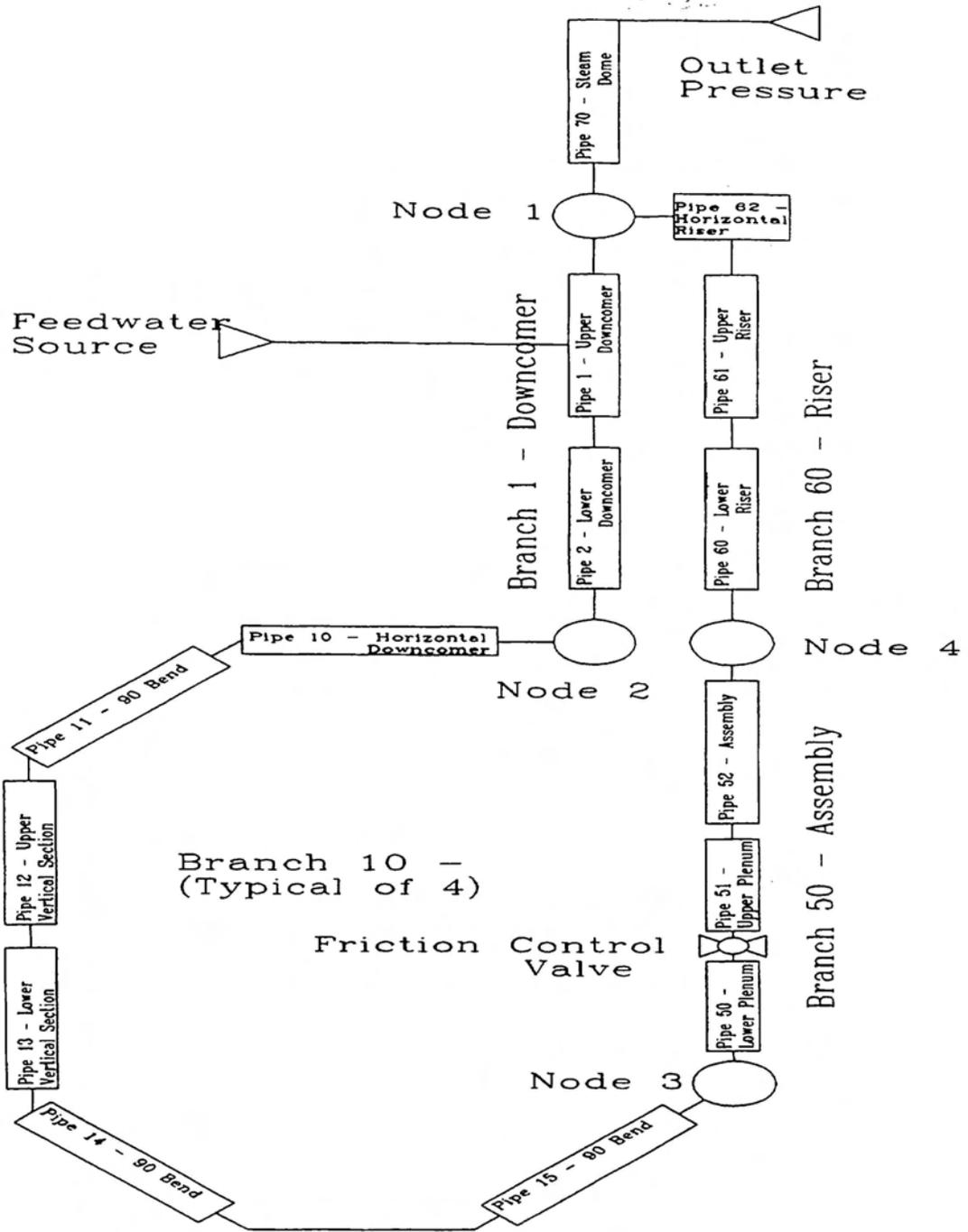
system, the ninety-degree bends in the downcomer loop piping, and the assembly spacers. The friction control valve was included directly. A cosine-shaped axial power distribution was input for the heated rods. No radial power distribution can be applied in the current model. The feedwater inlet temperature and flow rate and the steam dome outlet pressure are specified as boundary conditions.
