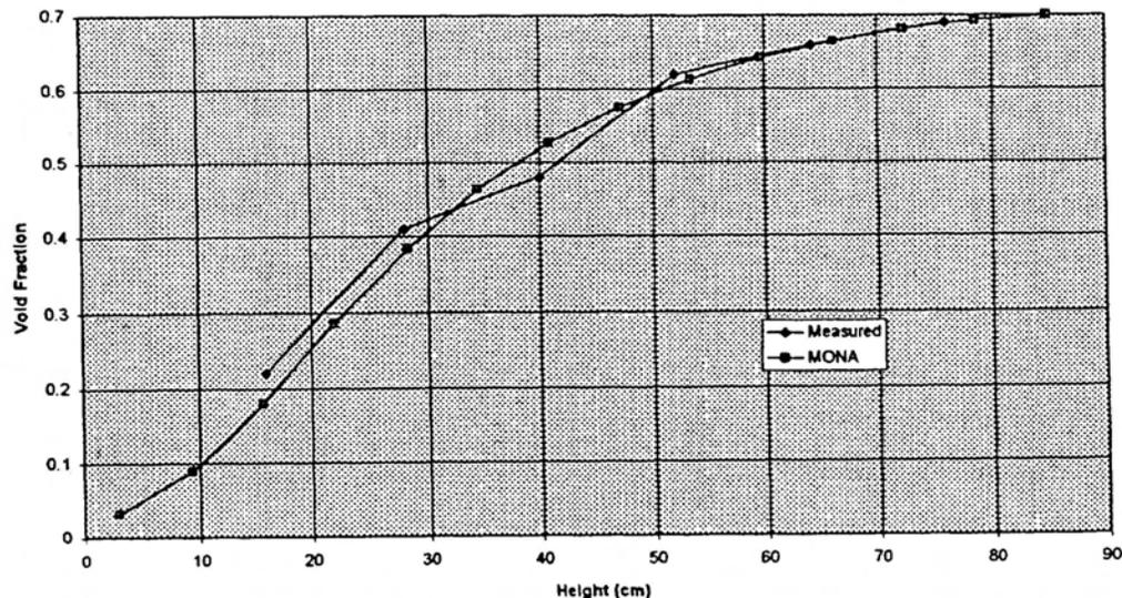
excellent agreement with the experimental data for this case. The measured axial void profile was obtained using the IRI gamma transmission tomography instrumentation.<sup>6</sup> In this device a gamma radiation beam is passed through the flow subchannel and the attenuated beam is measured on the opposite side. This provides an indication of the void fraction present in the subchannel because the vapor is less effective than the liquid in attenuating the radiation beam.
