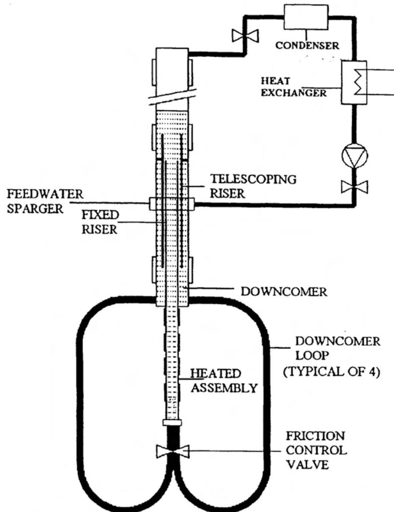
FIGURE 1 - DESIRE ASSEMBLY LAYOUT
