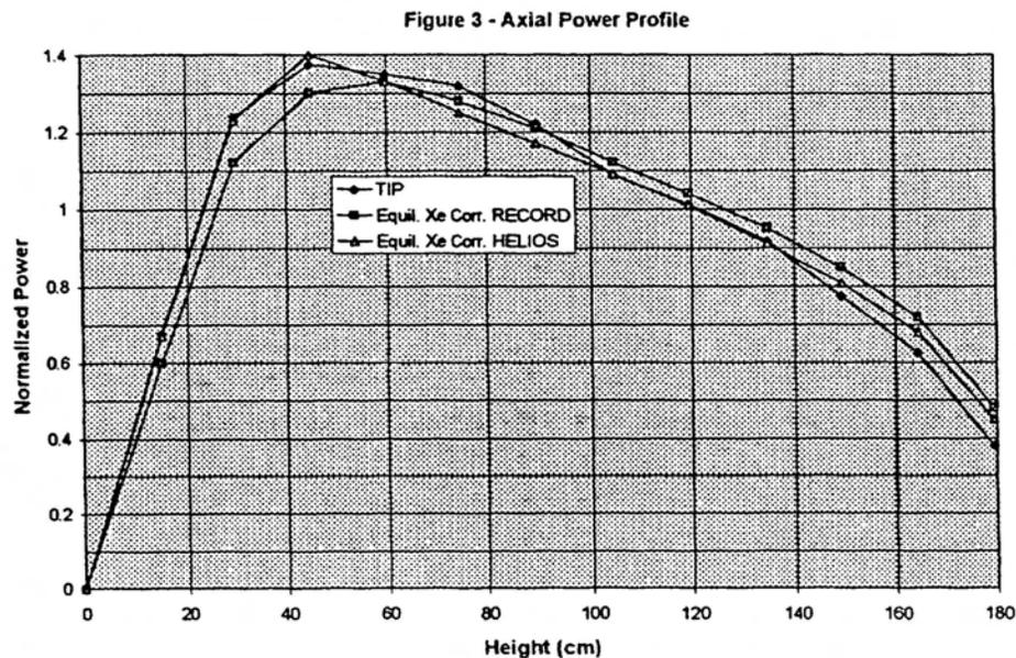
axial power profile predictions obtained with the HELIOS data show superior agreement with the measured TIP data relative to the results obtained using the RECORD libraries,
