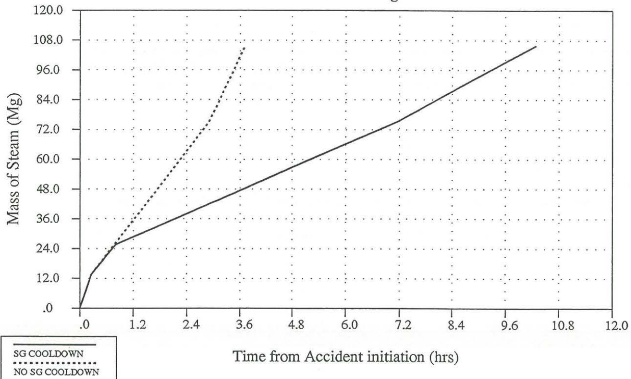
FIGURE 2: Steam Inventory in Containment during Blowdown
