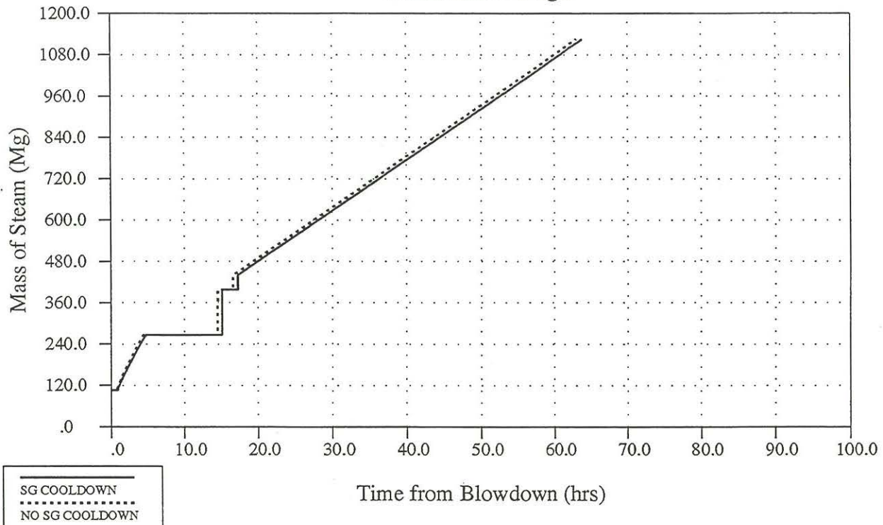
FIGURE 8: Steam Inventory in Containment during CDSs
