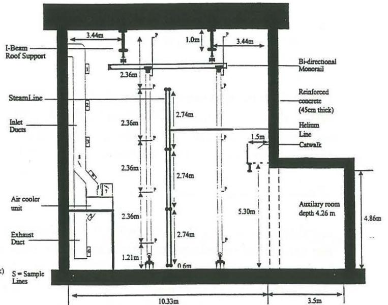
Figure 1: A schematic of the facility (a view of the east wall, from the west wall).
