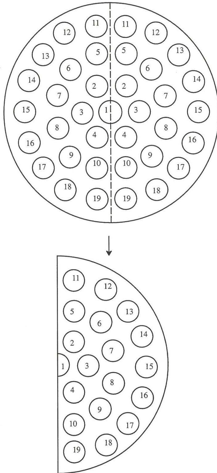
Figure 2. CATHENA detailed fuel modelling
