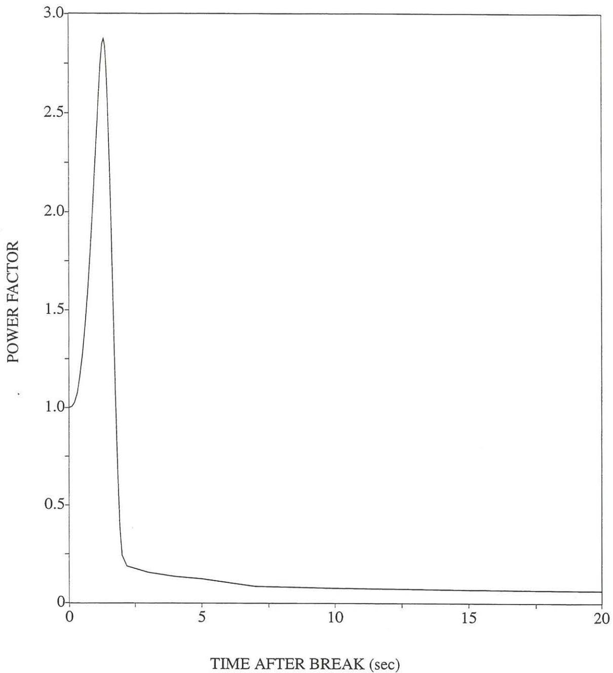
Figure 4. 7.3 MW channel power transient (20% RIH break with total loss of ECC), channel O17
