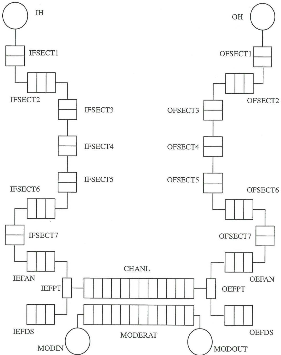
Figure 1. CATHENA thermalhydraulic node/link representation
