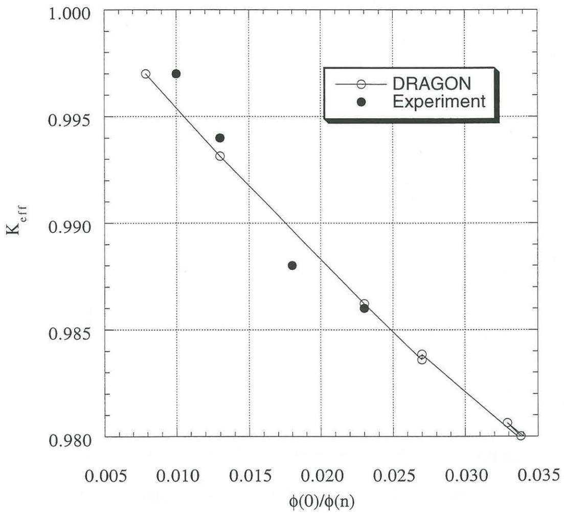
Figure 3:  $K_{\text{eff}}$  versus  $\phi(0)/\phi(n)$  for HEU core.
