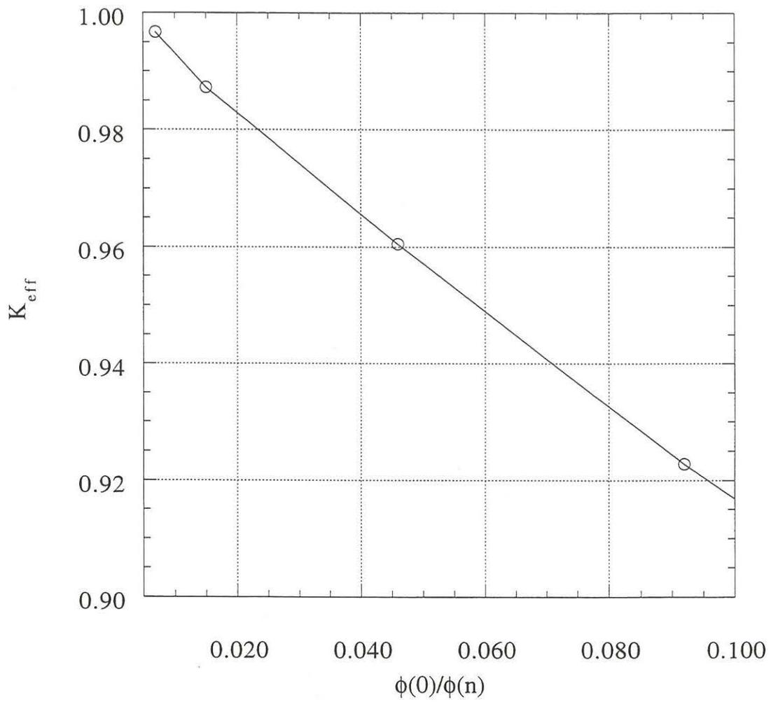
Figure 4:  $K_{\text{eff}}$  versus  $\phi(0)/\phi(n)$  for LEU core.
