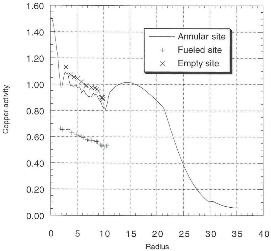
Figure 6: Radial distribution for the Copper activity in the LEU core.
