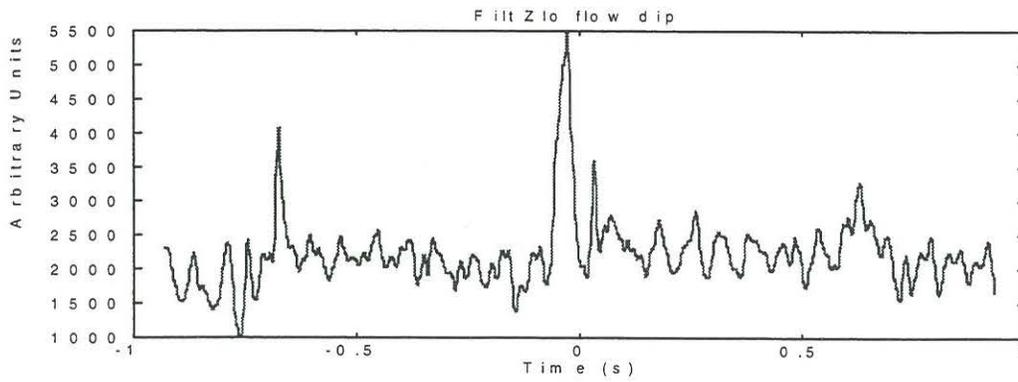
Figure 4e: Plot of FiltZlo, the envelope of the Zlo accelerometer response, near a flow dip.
