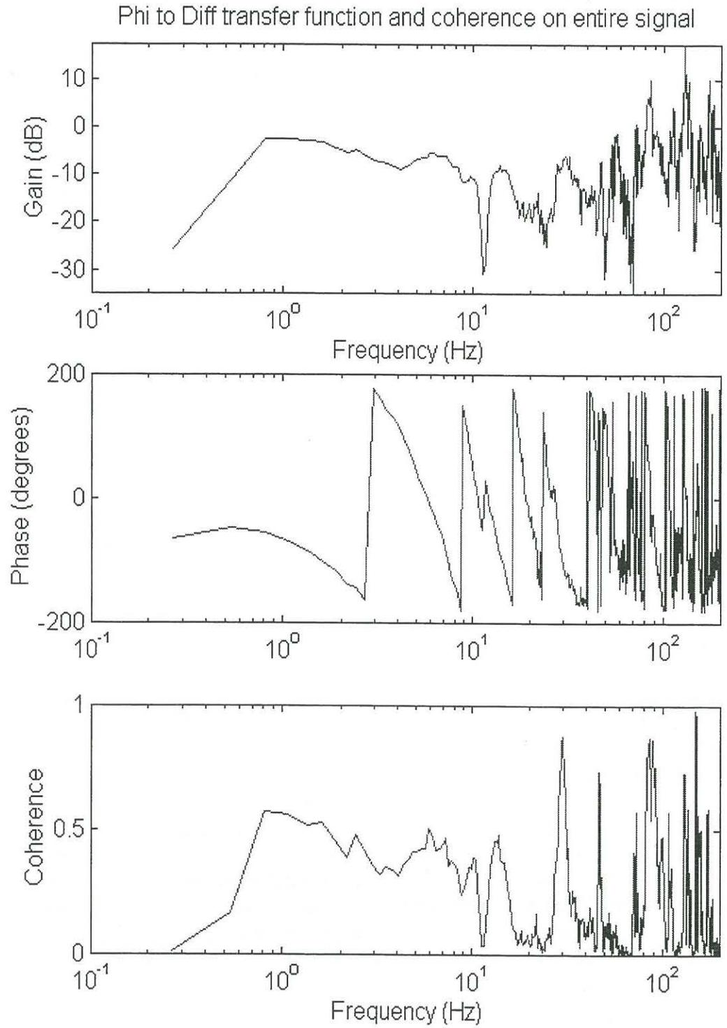
Figure 6: Phi to Diff transfer function.
