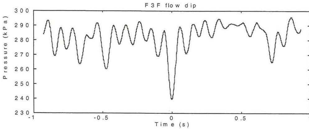
Figure 4a: Plot of F3F, the output of the standard PNGS B DP cell, near a flow dip.
