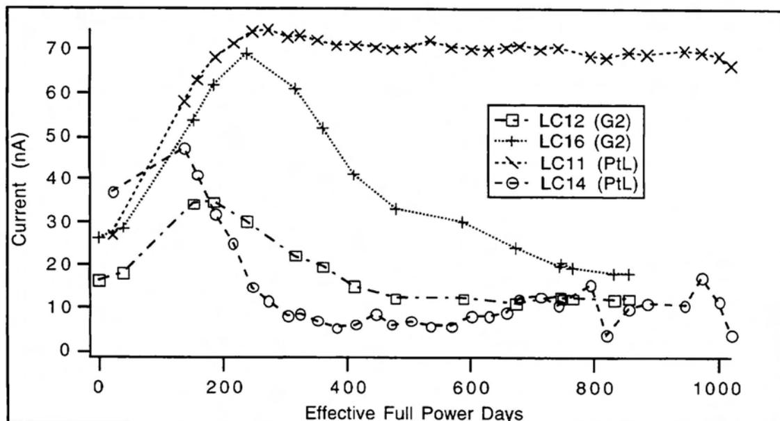
Figure 1: Measured Lead-cable Currents
