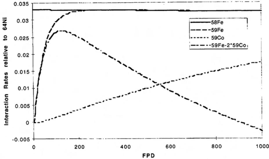
**Figure 5: Interaction Rates of  $^{58}\text{Fe}$ ,  $^{59}\text{Fe}$  and  $^{59}\text{Co}$  relative to  $^{64}\text{Ni}$  vs. FPD in Inconel 600**
