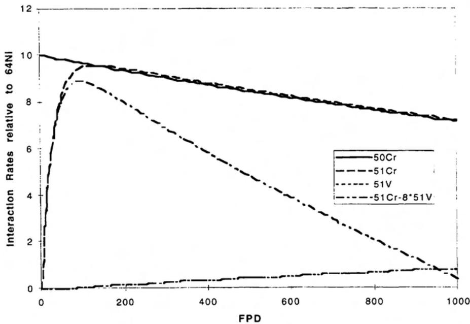
Figure 4: Interaction Rates of  $^{50}\text{Cr}$ ,  $^{51}\text{Cr}$  and  $^{51}\text{V}$  relative to  $^{64}\text{Ni}$  vs. FPD in Inconel 600
