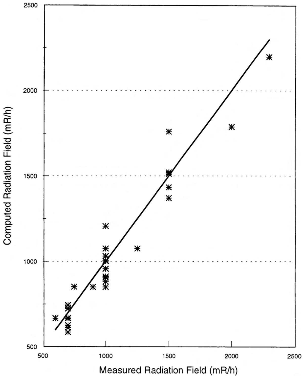
the drum exceeds 500 mR/h. The correlation is accurate enough to allow fine tuning of the liquid and bitumen emulsion flowrates. This ensures that the radiation field on any drum does not exceed about 3 R/h on contact.
