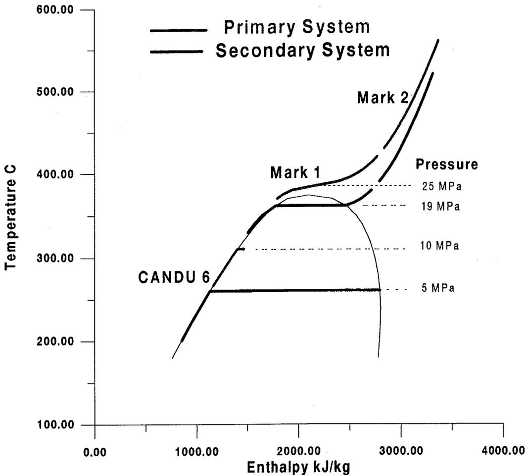
Figure 2: CANDU Evolution to Supercritical Coolant Conditions
