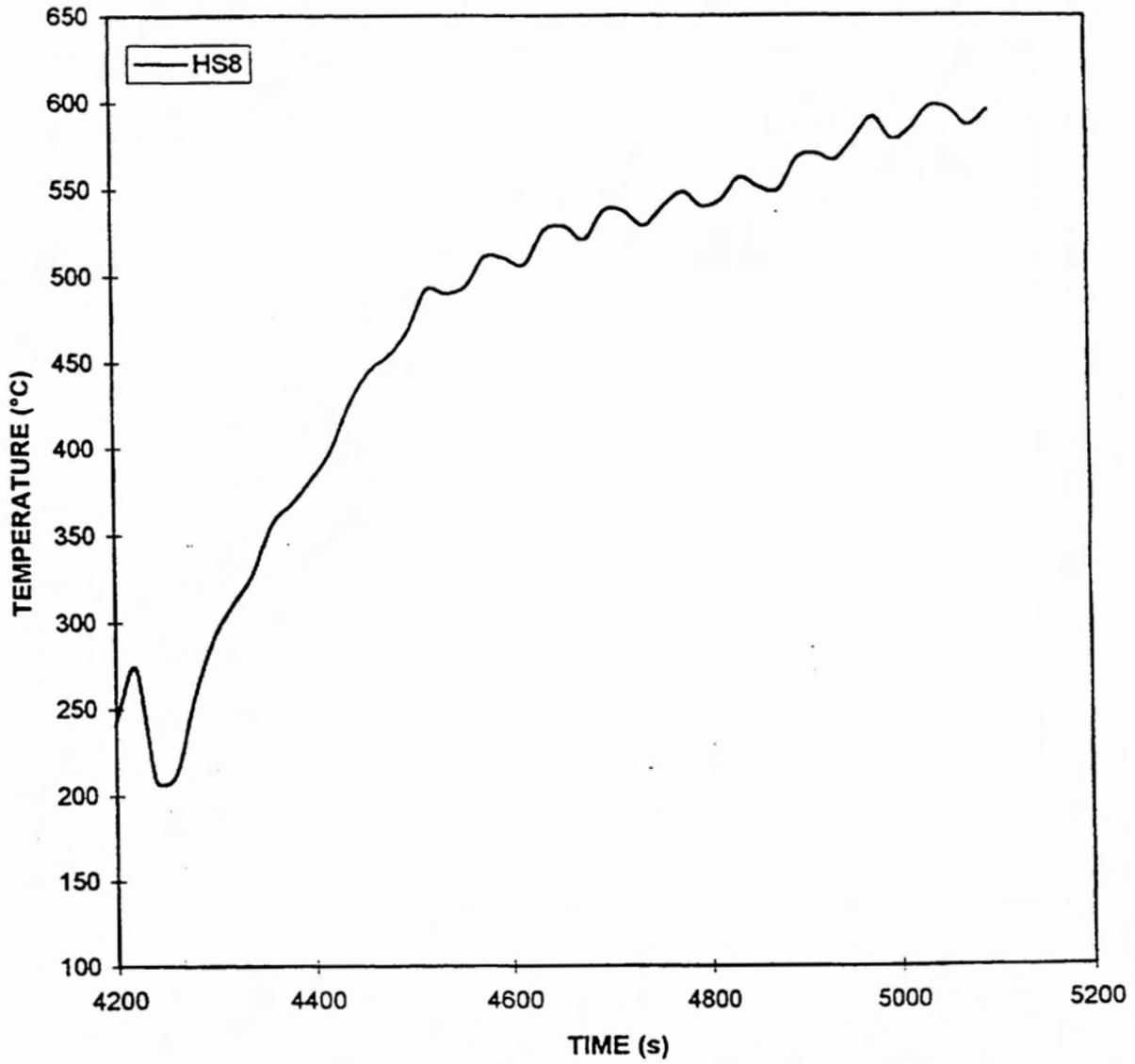
Figure 16 Peak FES Temperature Measured in Heated Section 8 in Test T8809.
