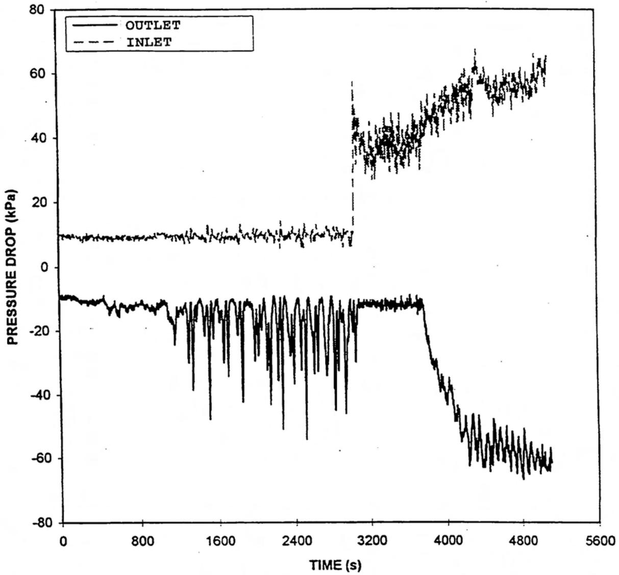
Figure 14 Inlet and Outlet Feeder Differential Pressure Measurements for Heated Section 8 in Test T8809.
