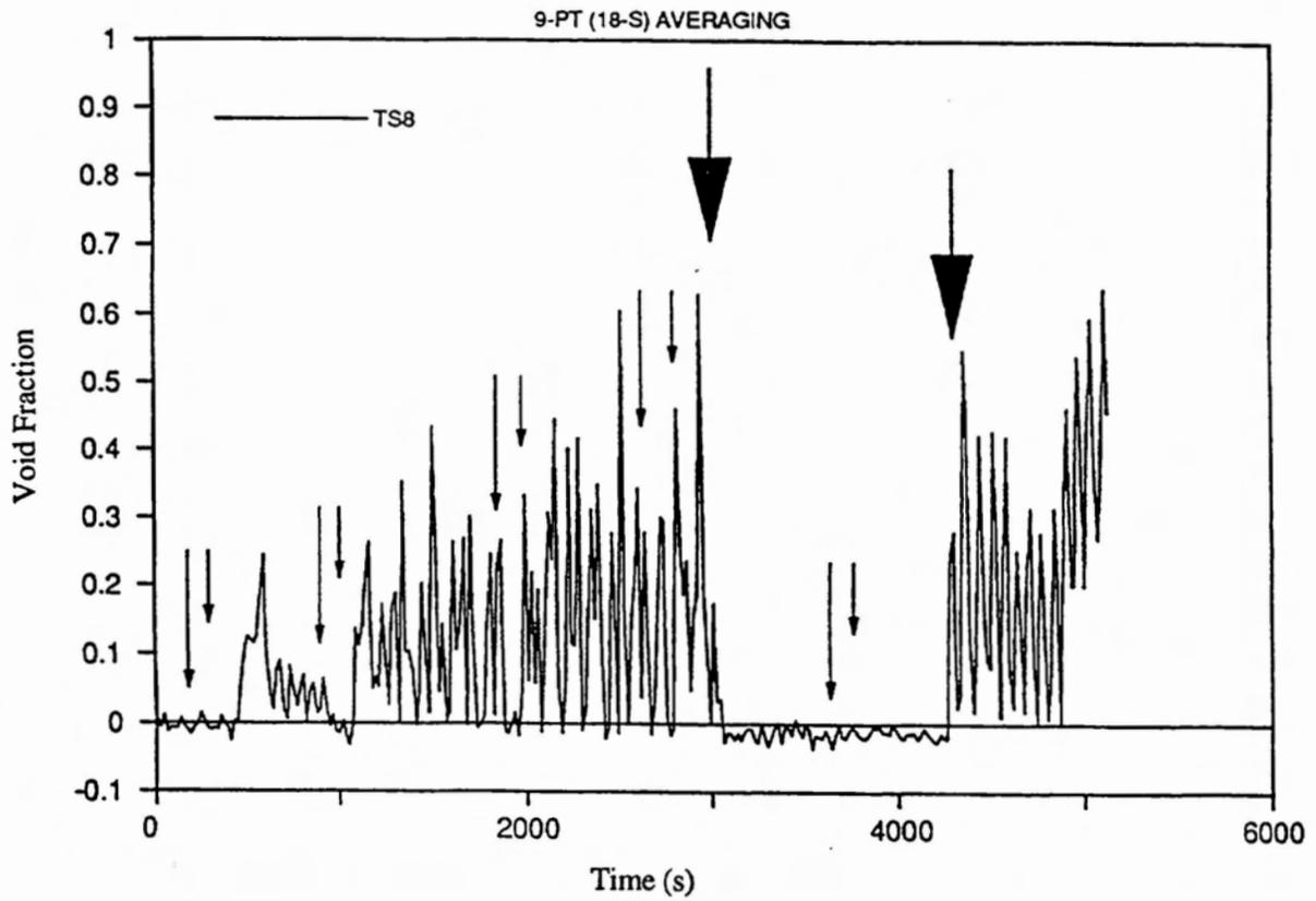
Figure 15 Void Fraction of Fluid Leaving Test Section 8 as a Function of Time in Test T8809.
