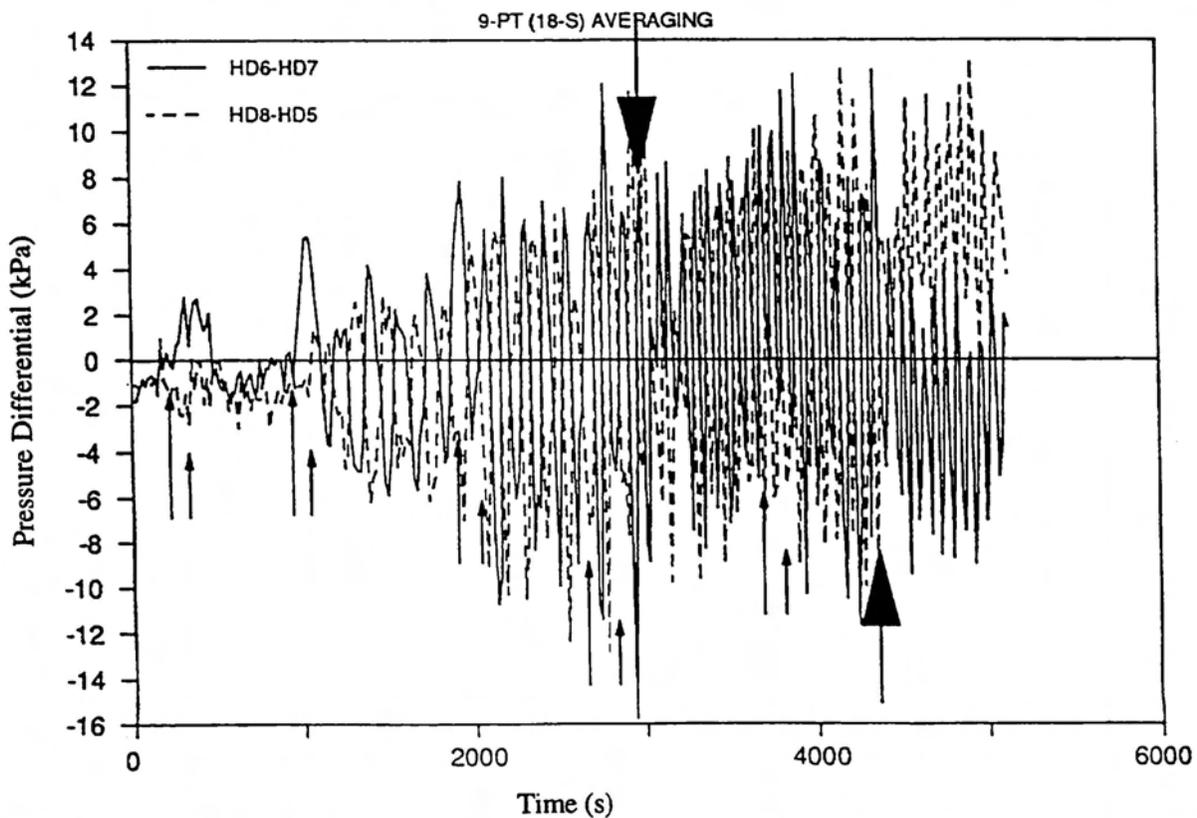
Figure 10 Header-to-Header Pressure Differential as a Function of Time in Test T8809
