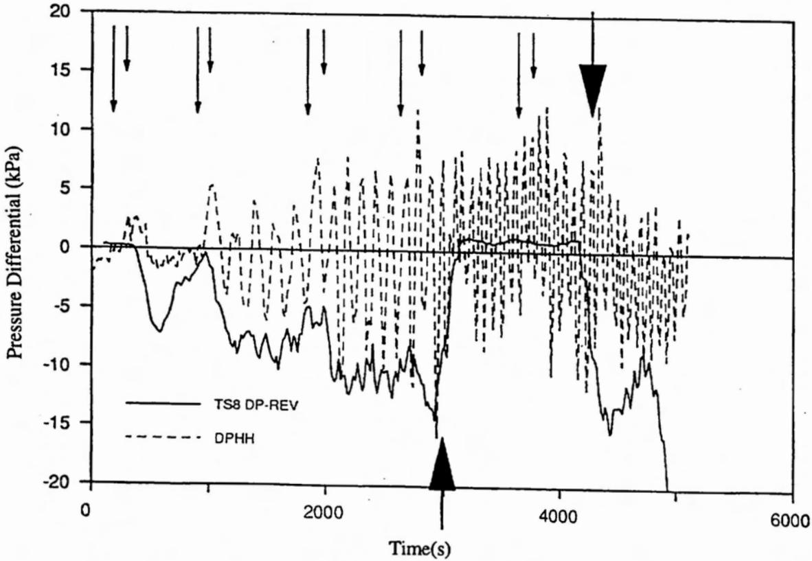
Figure 12 Comparison of Experimentally Measured Header-to-Header Pressure Differential (kPa) and the Header-to-Header Pressure Differential Required for Flow Reversal in Heated Section 8 in Test T8809.
