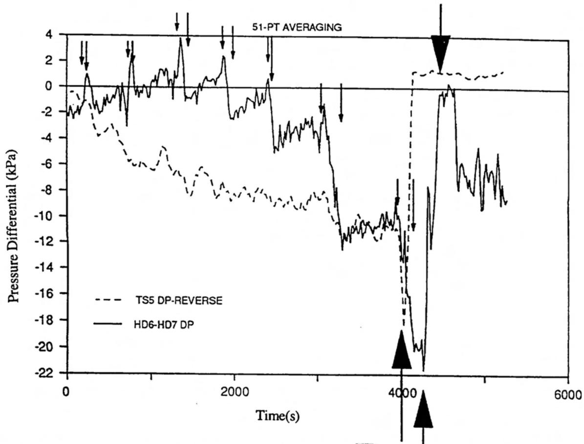
Figure 9 Comparison of Experimentally Measured Header-to-Header Pressure Differential and the Header-to-Header Pressure Differential Required to Flow Reversal in Heated Section 5 in Test T8805.
