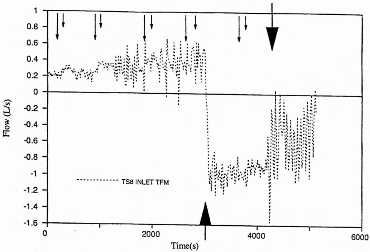
Figure 11 Inlet Feeder Turbine Flow Meter Reading Transient for Heated Section 8 in Test T8809.
