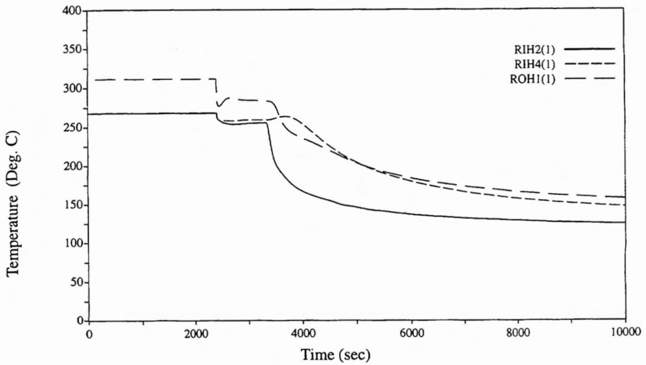
**Figure 15 Reactor Header Coolant Temperature For a SGTR With LCIVP And Continuous D<sub>2</sub>O Feed**
