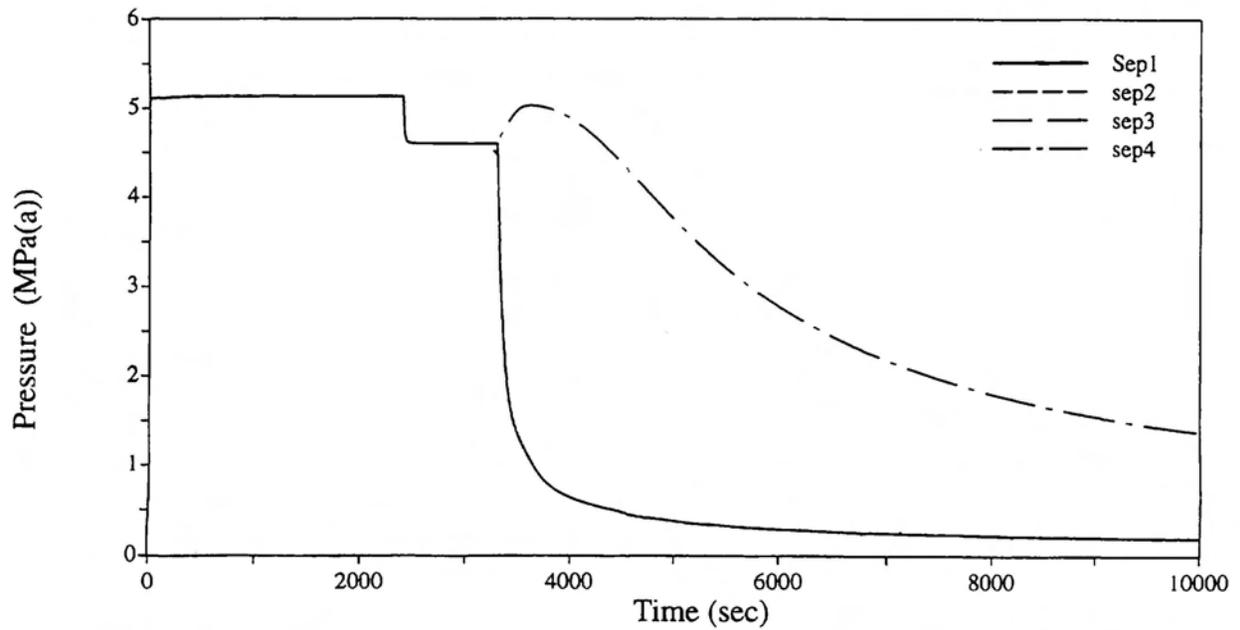
**Figure 14 Pressure Transients Of Boiler Separators For a SGTR With LCIVP And Continuous D<sub>2</sub>O Feed**
