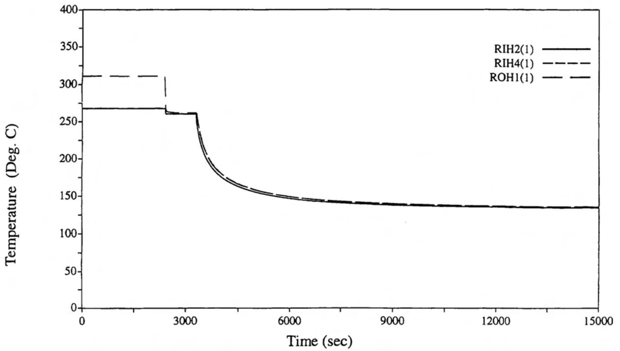
**Figure 7 Reactor Header Coolant Temperature With Continuous D<sub>2</sub>O Feed and No Additional Impairments**
