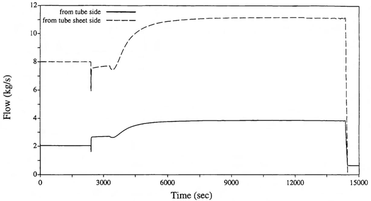
**Figure 5 Break Discharge Rates For SGTR With Continuous D<sub>2</sub>O Feed and No Additional Impairments**
