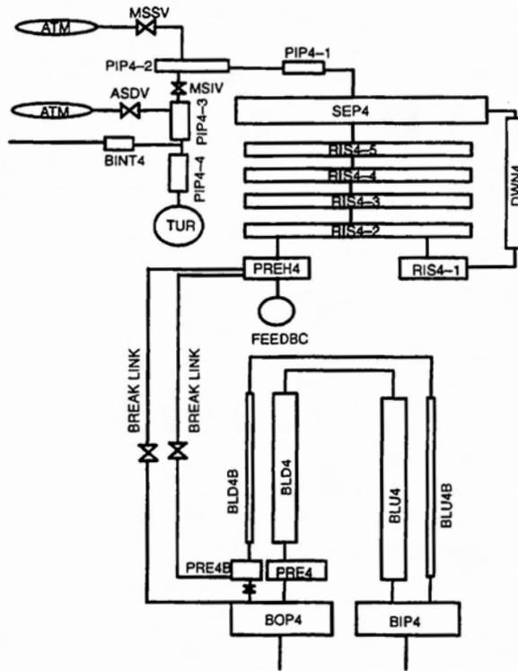
**Figure 3 Schematic Diagram of the Break Discharge Model**
