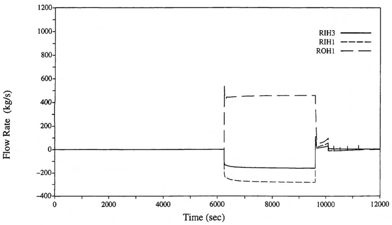
**Figure 10 ECCS Injection to the Headers For SGTR With Automatic Reactor Trip and No Additional Impairments**
