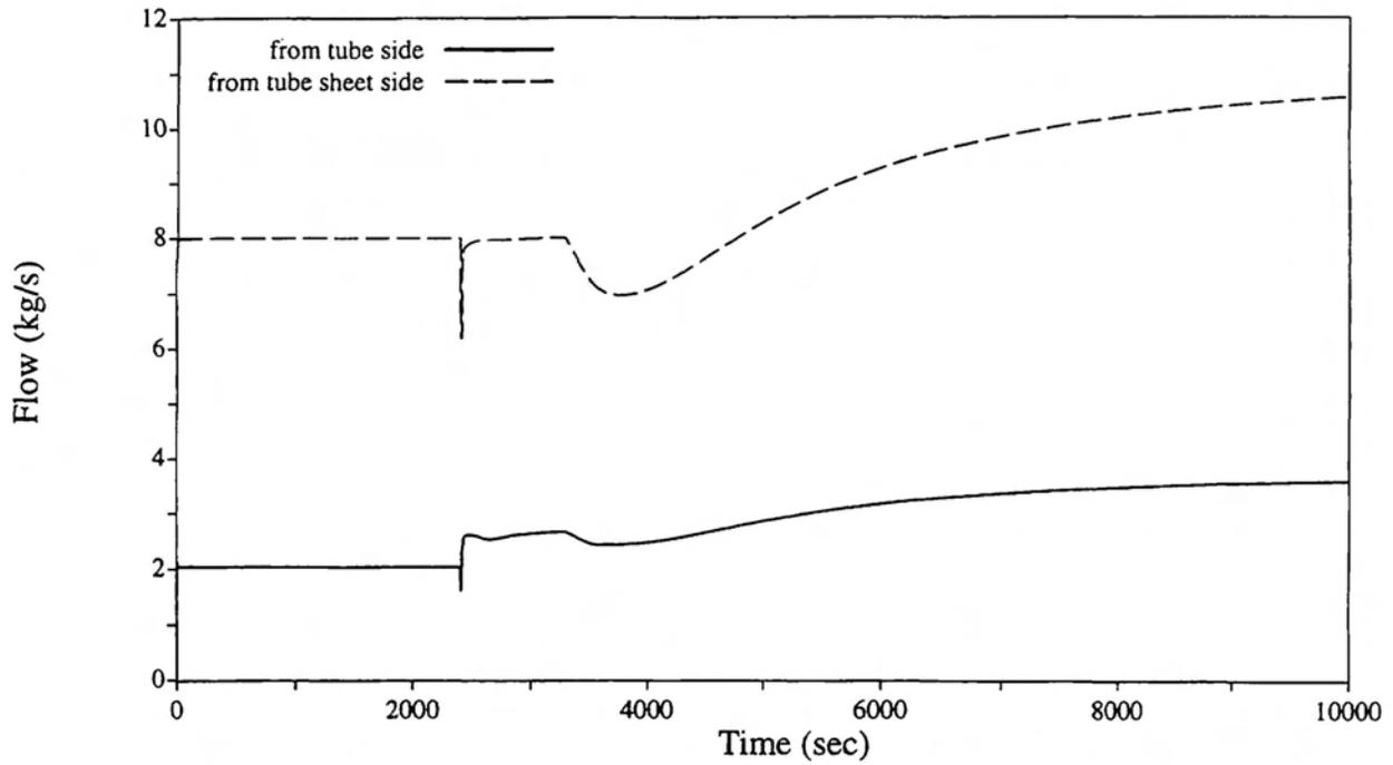
**Figure 13 Break Discharge For a SGTR With LCIVP And Continuous D<sub>2</sub>O Feed**
