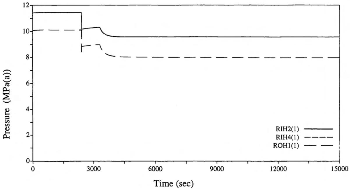
**Figure 6 Reactor Header Pressures For SGTR With Continuous D<sub>2</sub>O Feed and No Additional Impairments**
