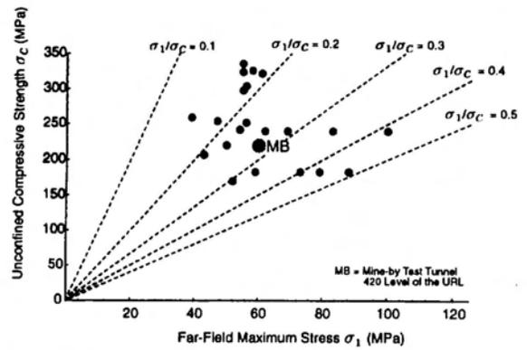
Figure 4: Empirical stability classification developed for square tunnels in South Africa.
