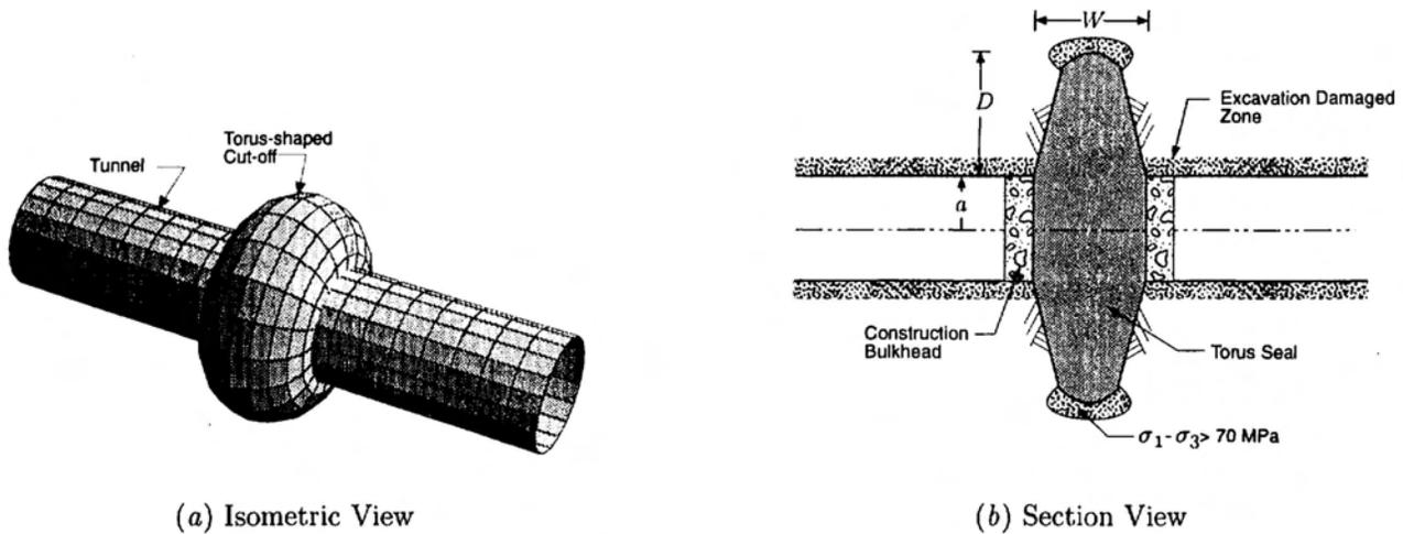
Figure 11: Illustration of a tunnel plug for a high stress environment using a torus concept as a cut-off.
