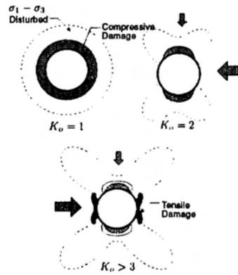
Figure 2: Relationship between damage and the disturbed zone for an unsupported circular opening in Region I in Figure 1.
