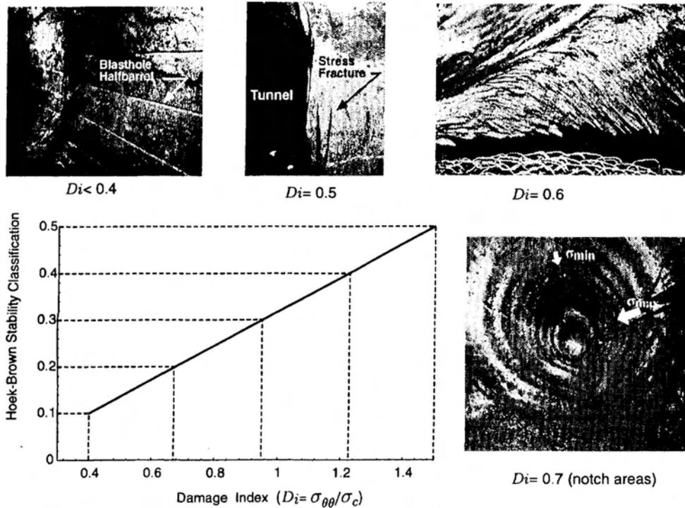
Figure 5: Damage index expressed as a function of the ratio between the maximum tangential boundary stress ( $\sigma_{\theta\theta}$ ) and the unconfined compressive strength ( $\sigma_c$ ).
