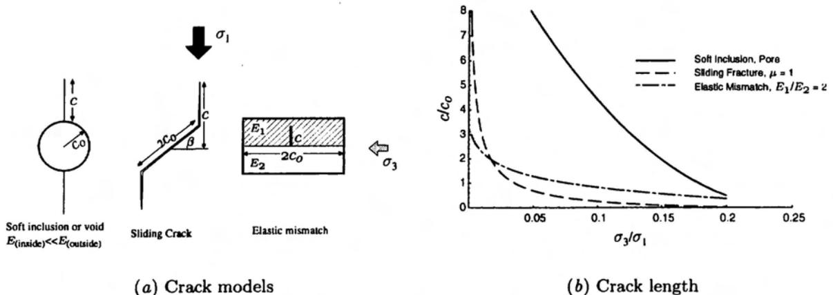
Figure 10: Crack models and crack extension as a function of  $\sigma_3/\sigma_1$ .
