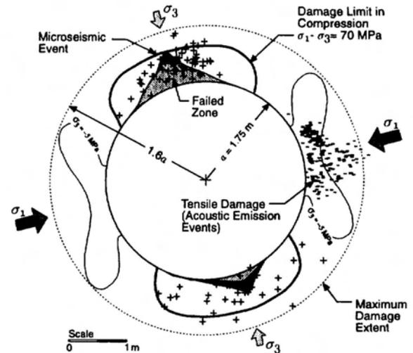
Figure 7: Extent and characteristics of excavation-induced damage around the Mine-by Experiment test tunnel ( $D_i = 0.7$  and  $K_o \approx 5$ ).
