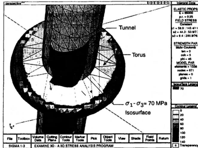
Figure 12: Numerical results from EXAMINE<sup>3D</sup> showing the effect of a torus-shaped seal as a cut-off to damage-initiation around the Mine-by test tunnel. The  $\sigma_1 - \sigma_3 = 70$  MPa isosurface is only calculated over the portion of the test tunnel close to the torus, and hence does not extend the full length of the tunnel in the figure.
