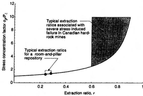
Figure 3: Stress concentrations in a pillar due to extraction ratio.
