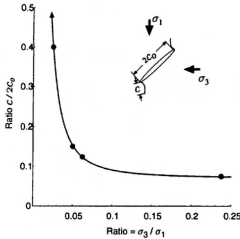
Figure 9: Relationship between crack propagation and the ratio of  $\sigma_3/\sigma_1$ , data from Hoek [8].
