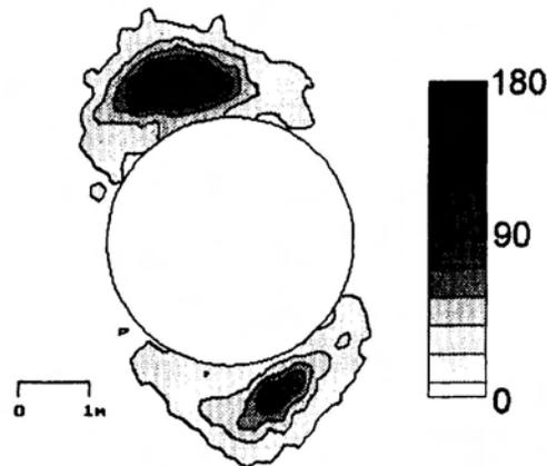
**Figure 4.** Spatial density of microseismic events recorded around the Mine-by tunnel during excavation [7].
