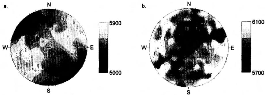
**Figure 1.** Lower hemisphere stereonet projections of P-wave velocity around the Mine-by tunnel in (a) the side wall of the tunnel and (b) the floor of the tunnel. The tunnel runs NE so the P-wave slow-velocity direction was perpendicular to the tunnel surface in both the side wall and floor of the tunnel.
