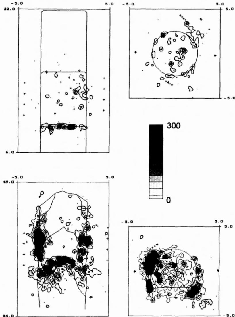
**Figure 6.** Spatial density plot of AE activity around the ZEDEX tunnels. The TBM tunnel is shown above and the D&B tunnel below with views are from above and looking along each tunnel.
