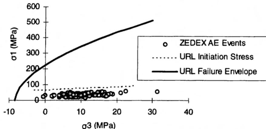
**Figure 7.** Crack initiation stress for ZEDEX AE events and fit to Mine-by microseismic events.
