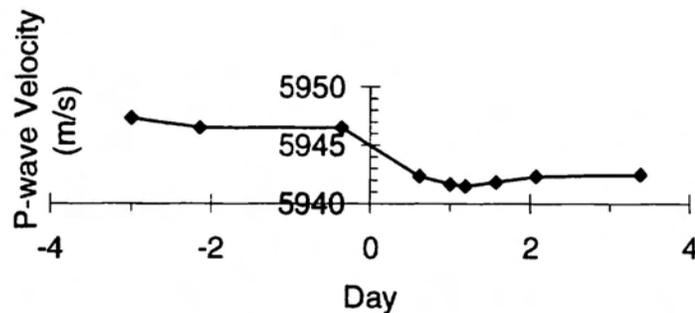
**Figure 3.** Variation in P-wave velocity with time as the TBM tunnel was excavated through the study volume. Time zero is the time when the TBM tunnel face passed through the centre of the sensor array. During the period shown about 25 m were excavated, approximately centred at the centre of the sensor array.
