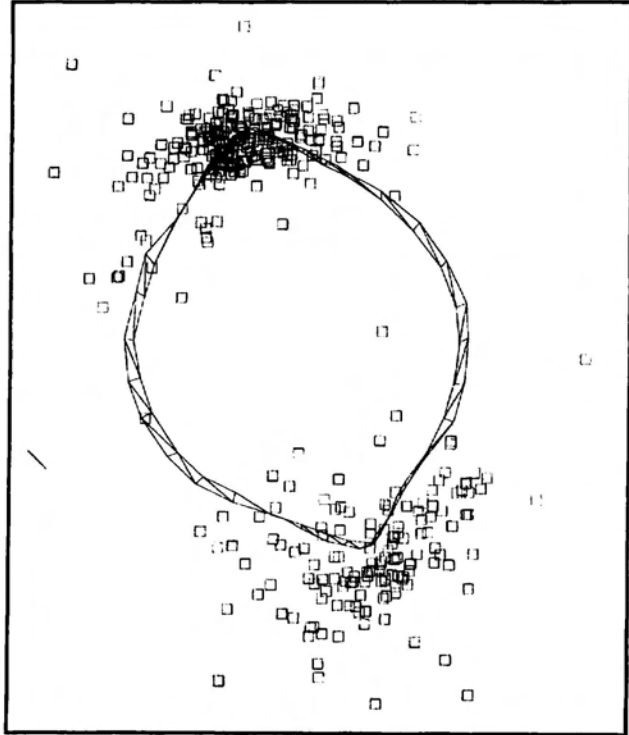
Figure 2. Axial view of the tunnel (3.5 m original diameter) showing the induced seismicity.
