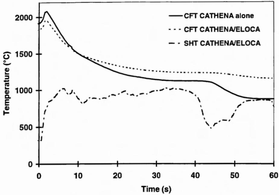
**Figure 4:** 20% RIH Break using CATHENA/ELOCA and CATHENA Alone - Centreline Fuel Temperature and Sheath Temperature for Top Outer Pin of Bundle 7
