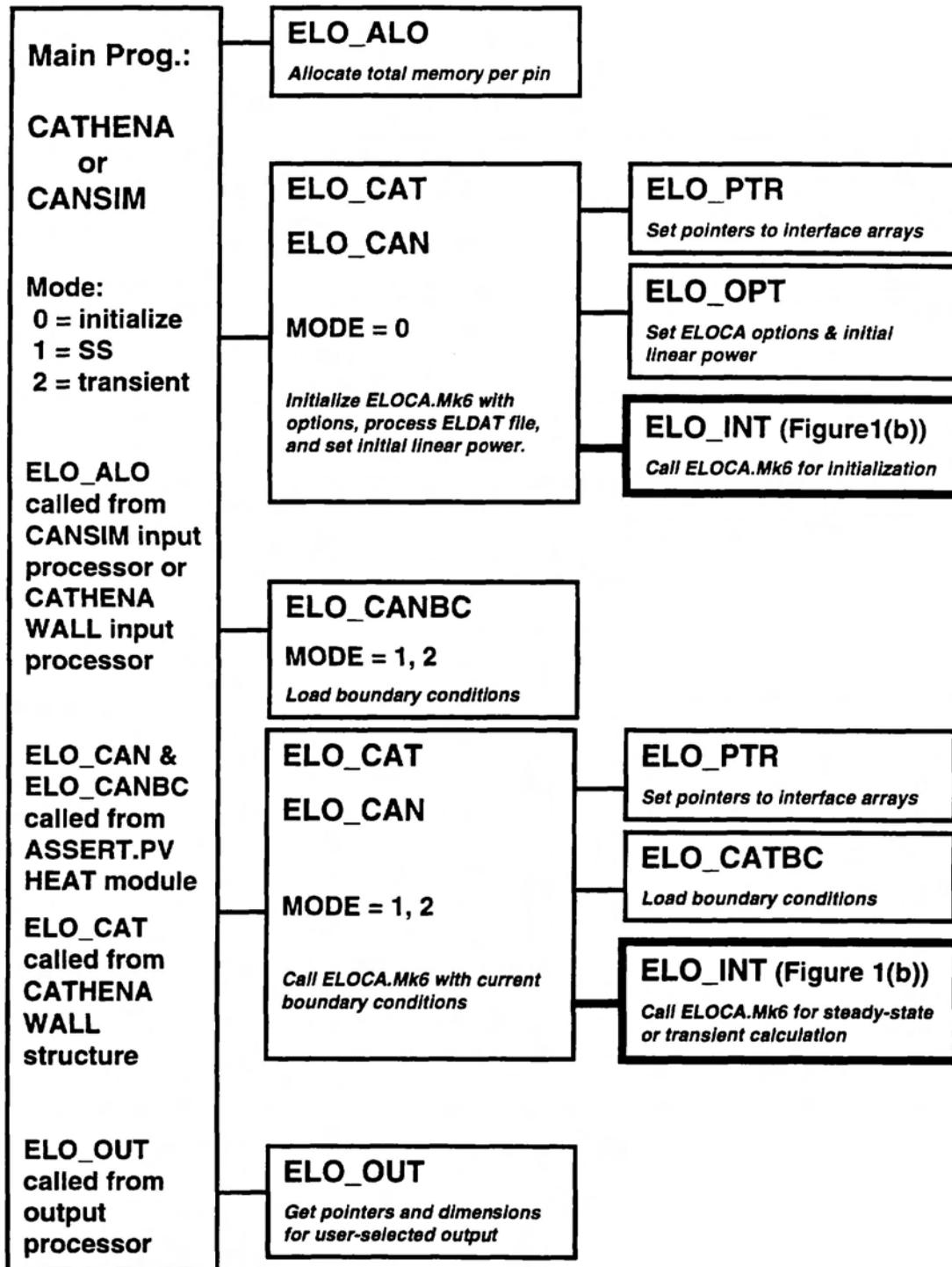
**Figure 1(a):** Coupling Architecture for CATHENA/ELOCA and CANSIM/ELOCA
