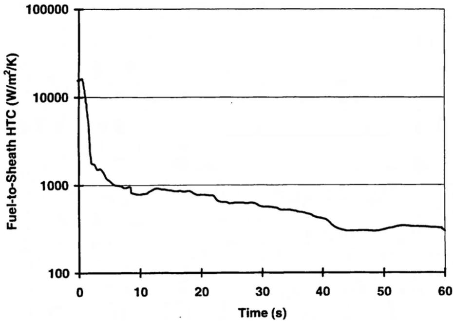
**Figure 3:** 20% RIH Break using CATHENA/ELOCA - Fuel-to-Sheath Heat Transfer Coefficient for Top Outer Pin of Bundle 7
