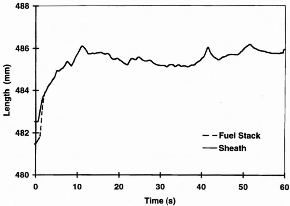
**Figure 5:** 20% RIH Break using CATHENA/ELOCA - Fuel Stack Length and Sheath Length for Top Outer Pin of Bundle 7
