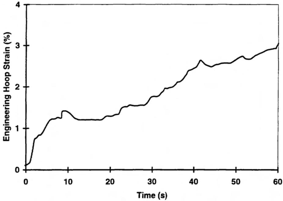
**Figure 2:** 20% RIH Break using CATHENA/ELOCA - Engineering Hoop Strain for Top Outer Pin of Bundle 7
