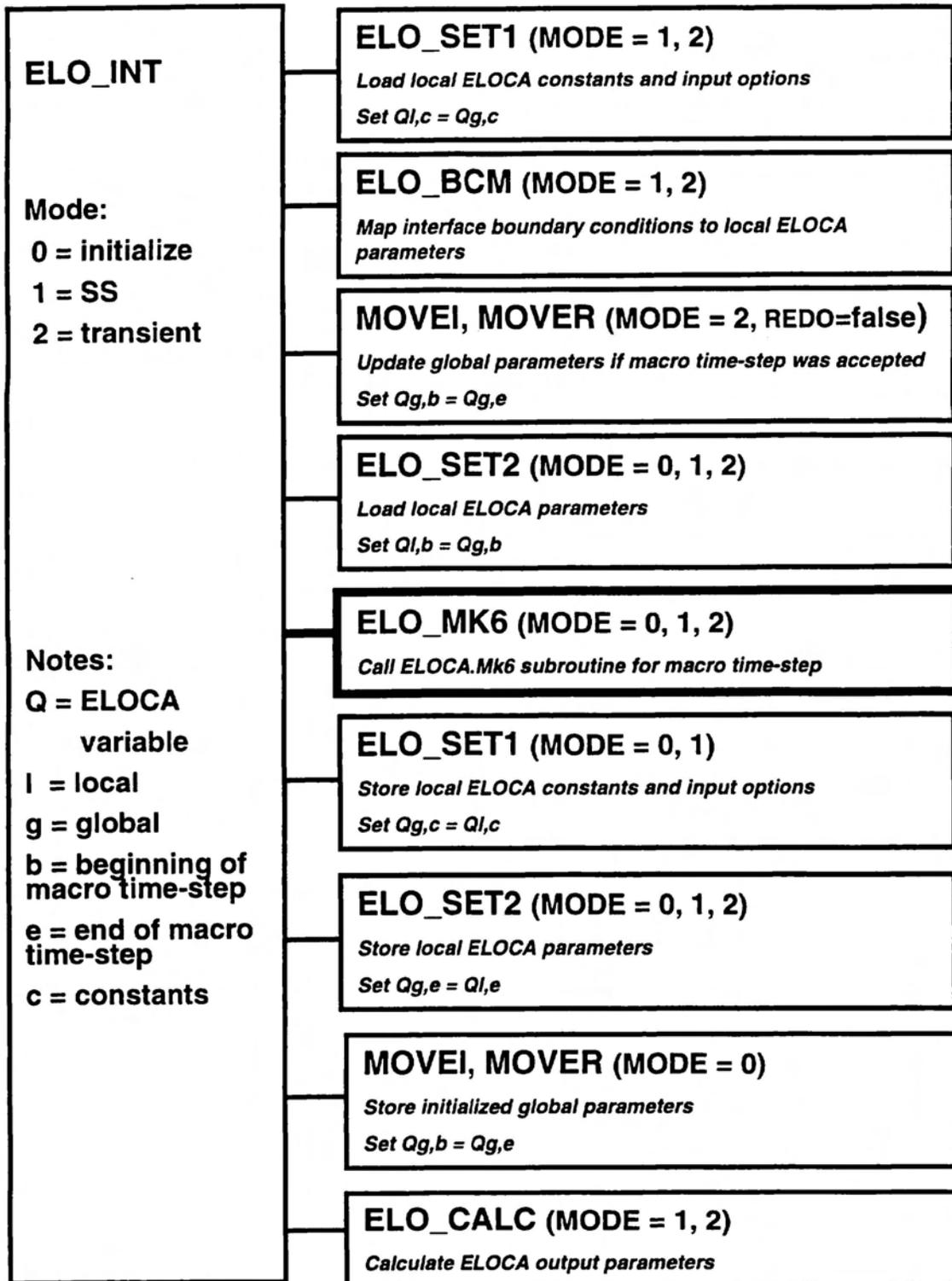
Figure 1(b): ELOCA.Mk6 Interface Architecture
