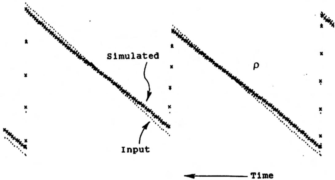
The last step in the analysis is to estimate the reactivity values that would have been measured if the gamma signal had not been present. These are simply the input reactivity values used in the simulation to match the observed flux behavior.
