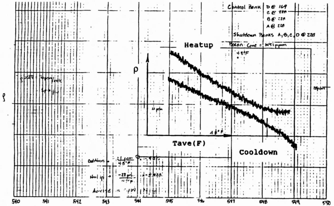
FIGURE 8 Anomalies During Rod Worth Measurements
