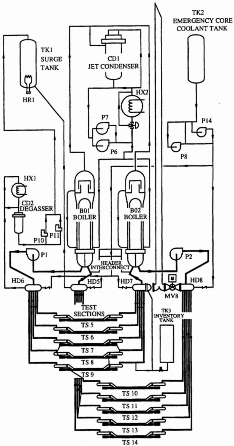
FIGURE 3: Schematic of RD-14M Facility
