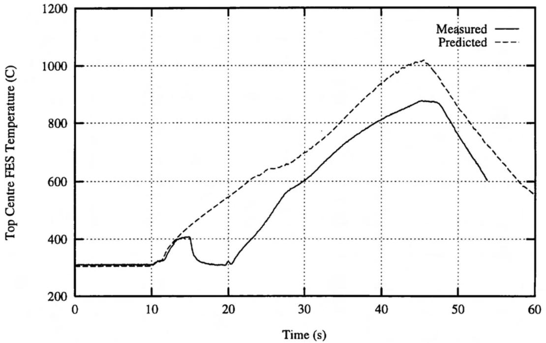
FIGURE 13: B9605 Post Test Simulation with Default Film Boiling Correlation
