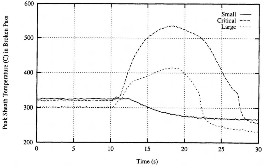
FIGURE 1: RD-14M Temperature Transients for Small, Large and Critical Breaks
