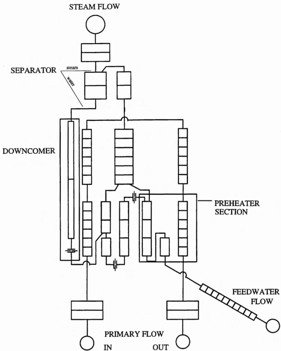
FIGURE 5: CATHENA Idealisation of RD-14M Secondary Side
