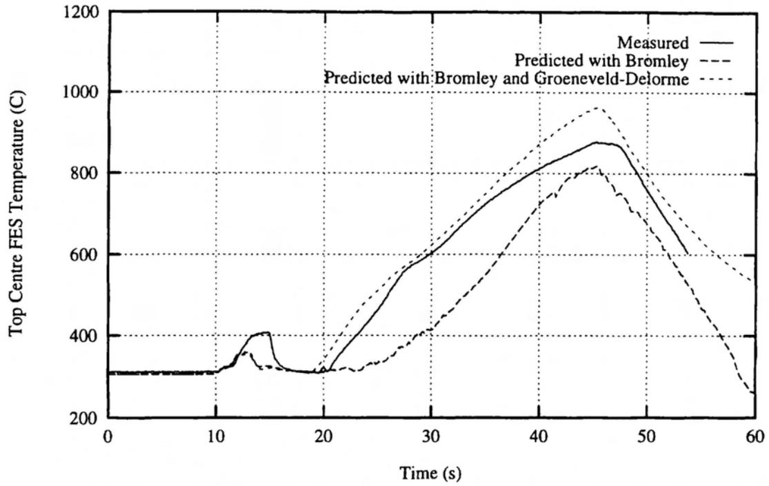
FIGURE 14: B9605 Post-Test Simulation with Bromley Correlation and with Combined Bromley and Default Correlations
