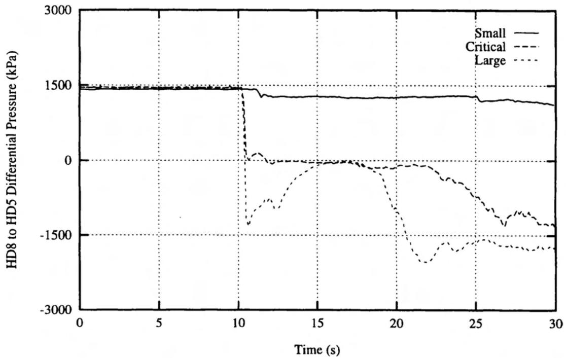
FIGURE 2: RD-14M Pressure Transients for Small, Large and Critical Breaks
