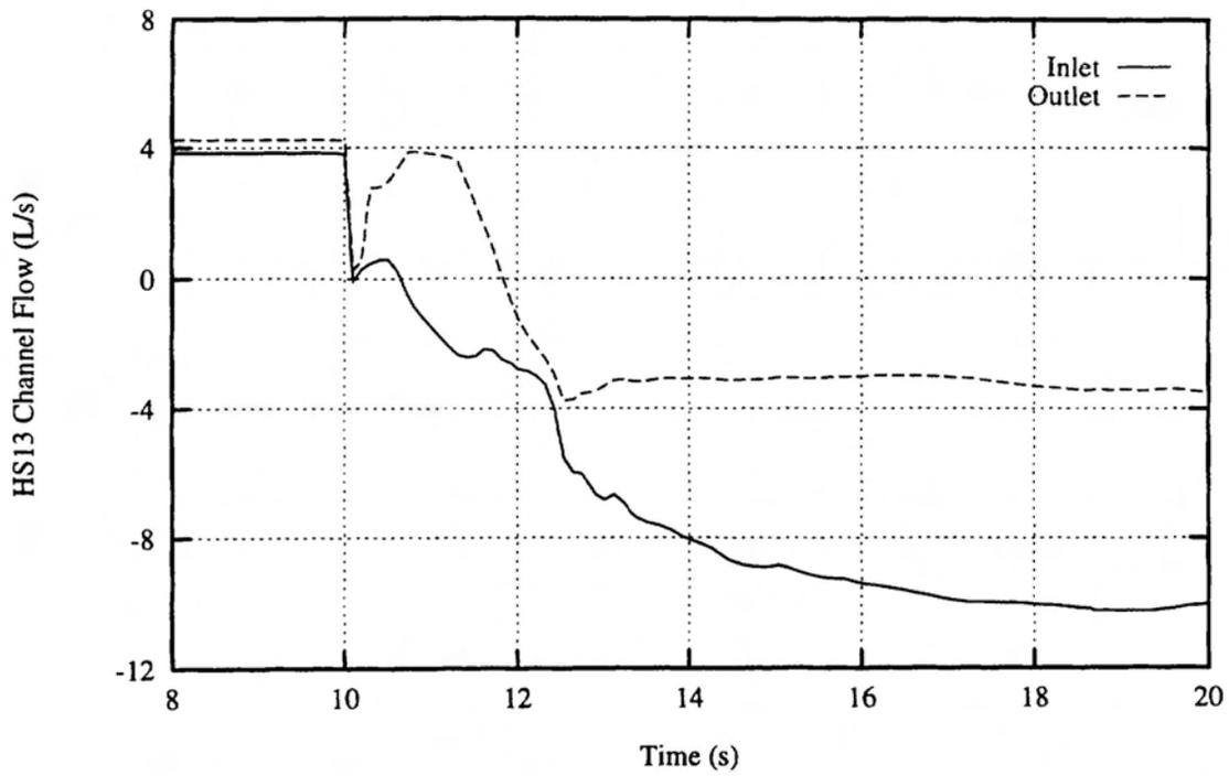
FIGURE 6: Break Size Scoping - 18 mm Break with 55% Pump Speed
