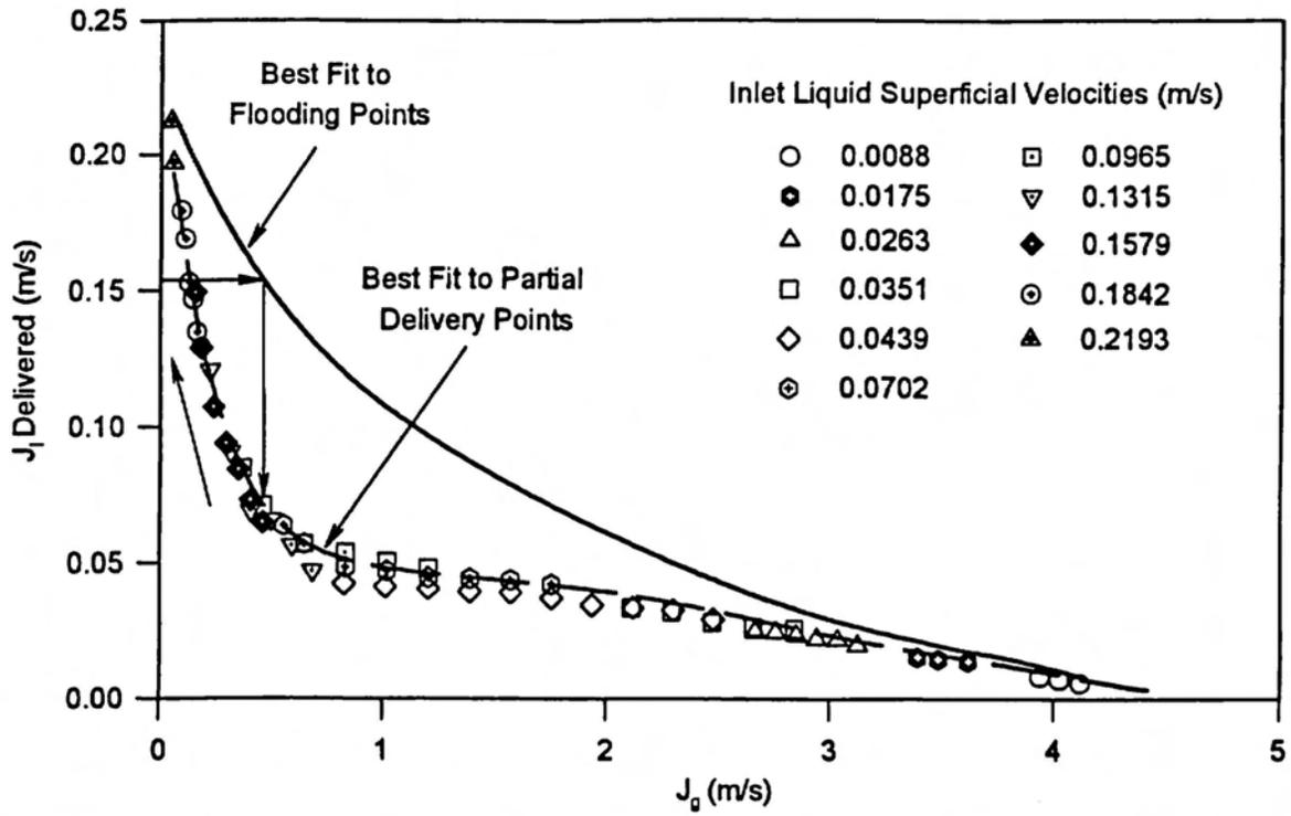
Figure 5c. Partial Delivery Results with Decreasing Gas Flow, Orifice  $\beta=0.77$  at Position 1.
