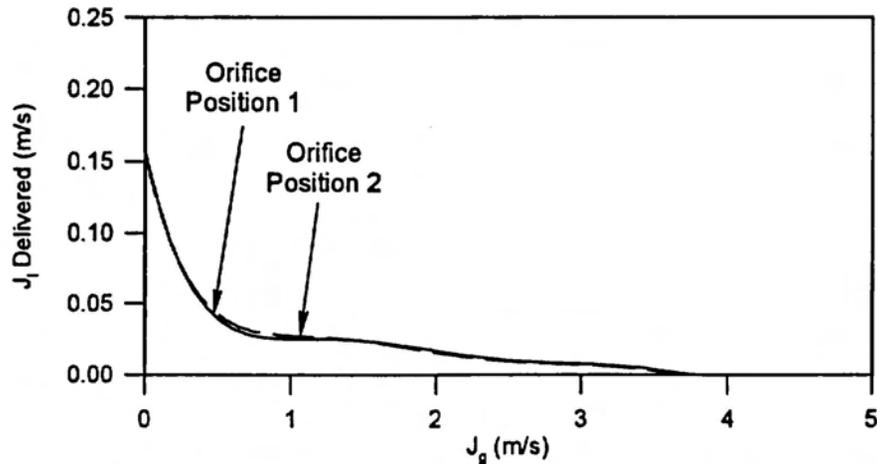
Figure 3c. Best Fit of  $J_1$  Delivered vs.  $J_g$  (Orifice  $\beta=0.66$  at Positions 1 & 2).
