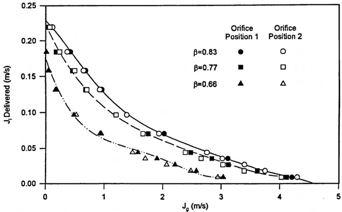
Figure 4b. Comparison of Flooding Points, Orifice Positions 1 & 2 ( $\beta=0.83$ , 0.77 and 0.66).
