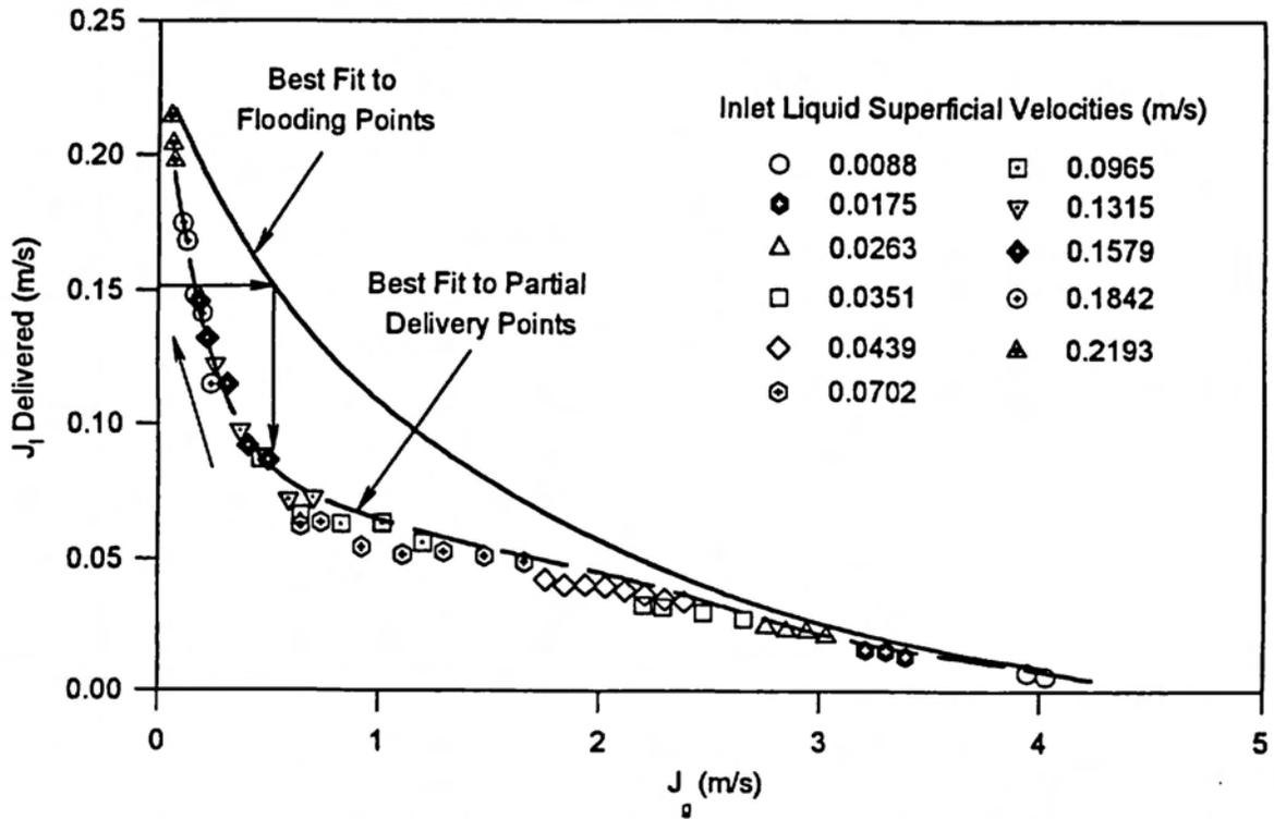
Figure 5d. Partial Delivery Results with Decreasing Gas Flow, Orifice  $\beta=0.77$  at Position 2.
