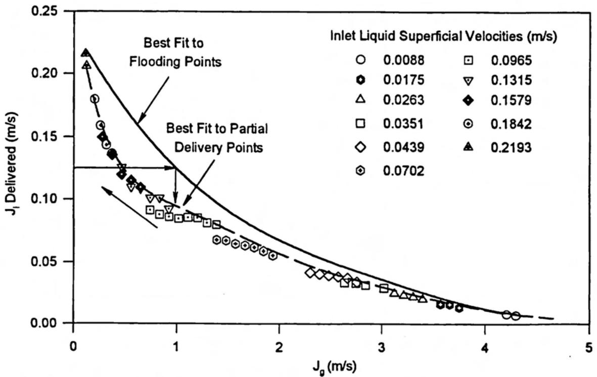
Figure 5b. Partial Delivery Results with Decreasing Gas Flow, Orifice  $\beta=0.83$  at Position 2.
