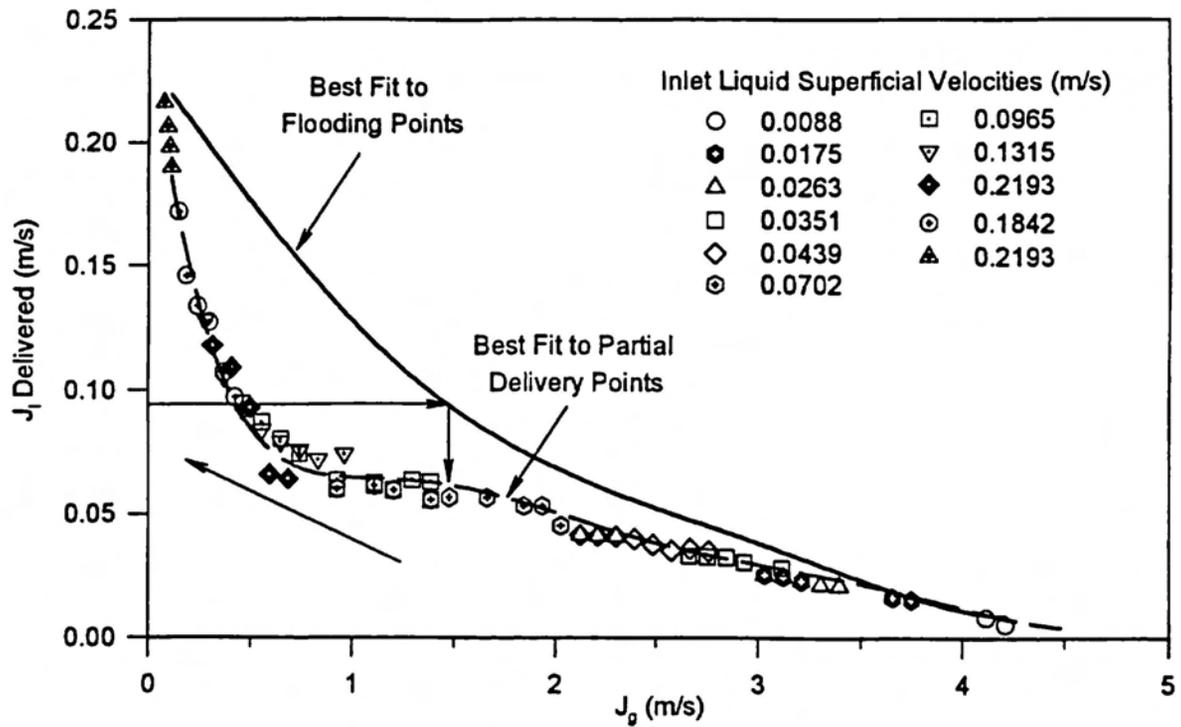
Figure 5a. Partial Delivery Results with Decreasing Gas Flow, Orifice  $\beta=0.83$  at Position 1.
