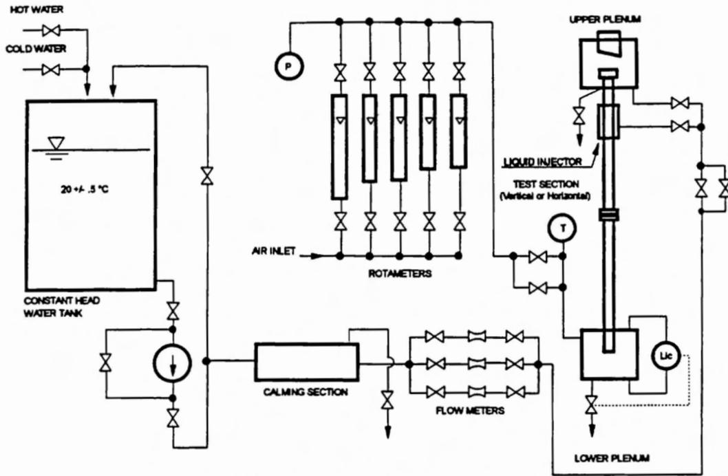
Figure 1. CCF Test Facility.
