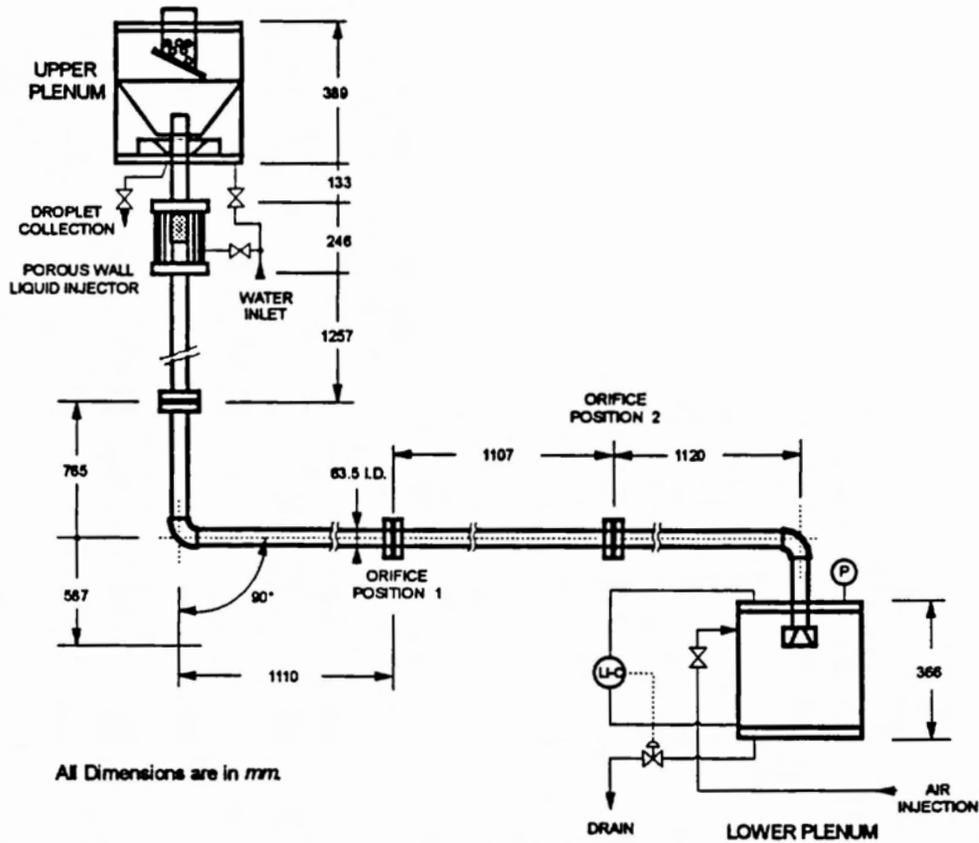
Figure 2. Test Section with Vertical and Horizontal Runs with Two Orifice Positions.
