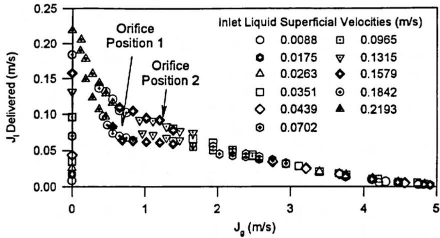
Figure 3a.  $J_1$  Delivered vs  $J_g$  ( $\beta=0.83$ , Orifice Position 1 & 2).
