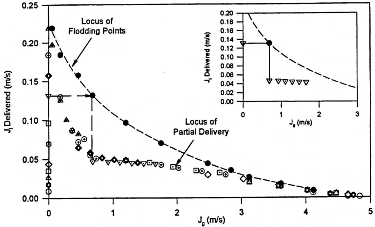
Figure 4a.  $J_l$  Delivered vs  $J_g$  and Flooding Points, Orifice  $\beta=0.77$  Located at Position 1.
