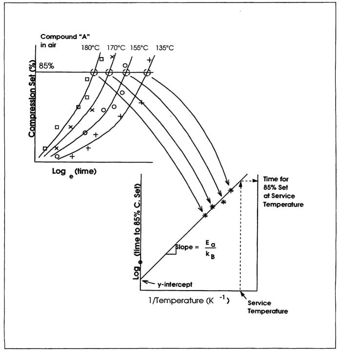
Figure 1: Arrhenius Thermal Aging Tests. This figure illustrates the number of points required for a reasonable extrapolation.
