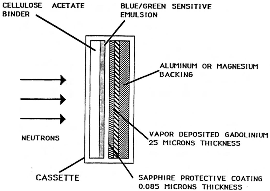
Figure 8. Example of film neutron radiography.
