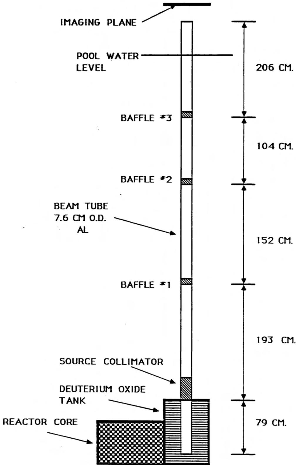
Figure 5. Cross section of the vertical neutron radiography port.
