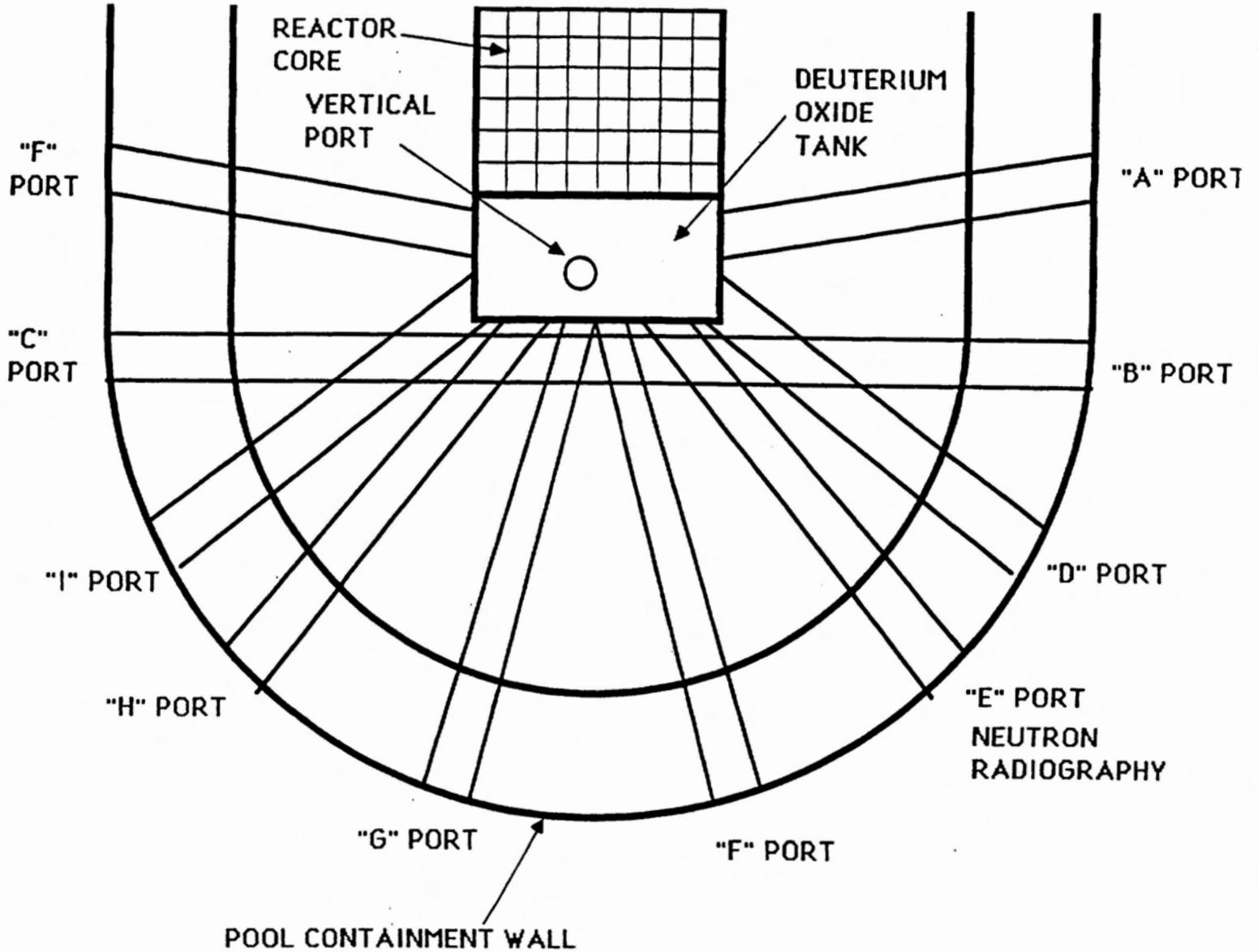
Figure 2. Cross section of FNR showing the reactor core, the deuterium oxide tank, and the beam ports.
