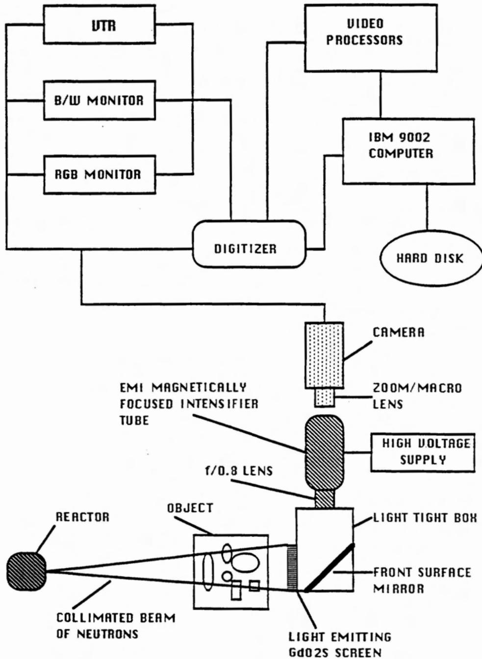
Figure 7. Schematic representation of the EMI neutron radiography imaging system.
