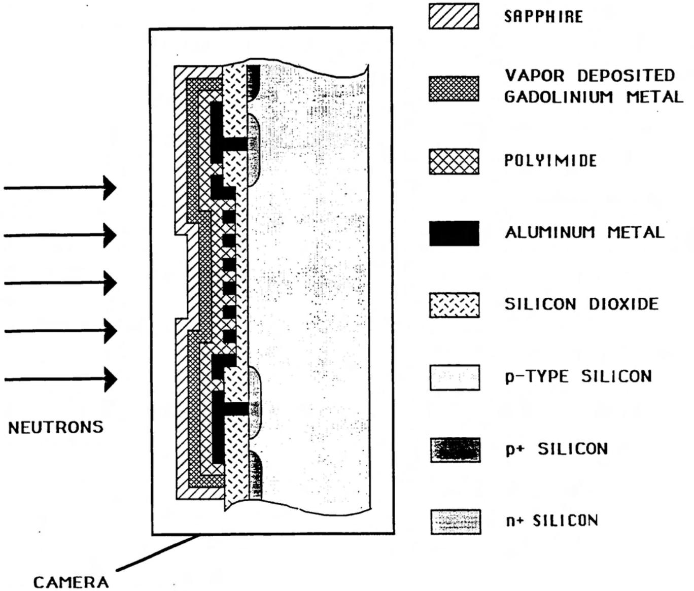
Figure 12. Generic example of a future neutron radiography device incorporating CCD technology.
