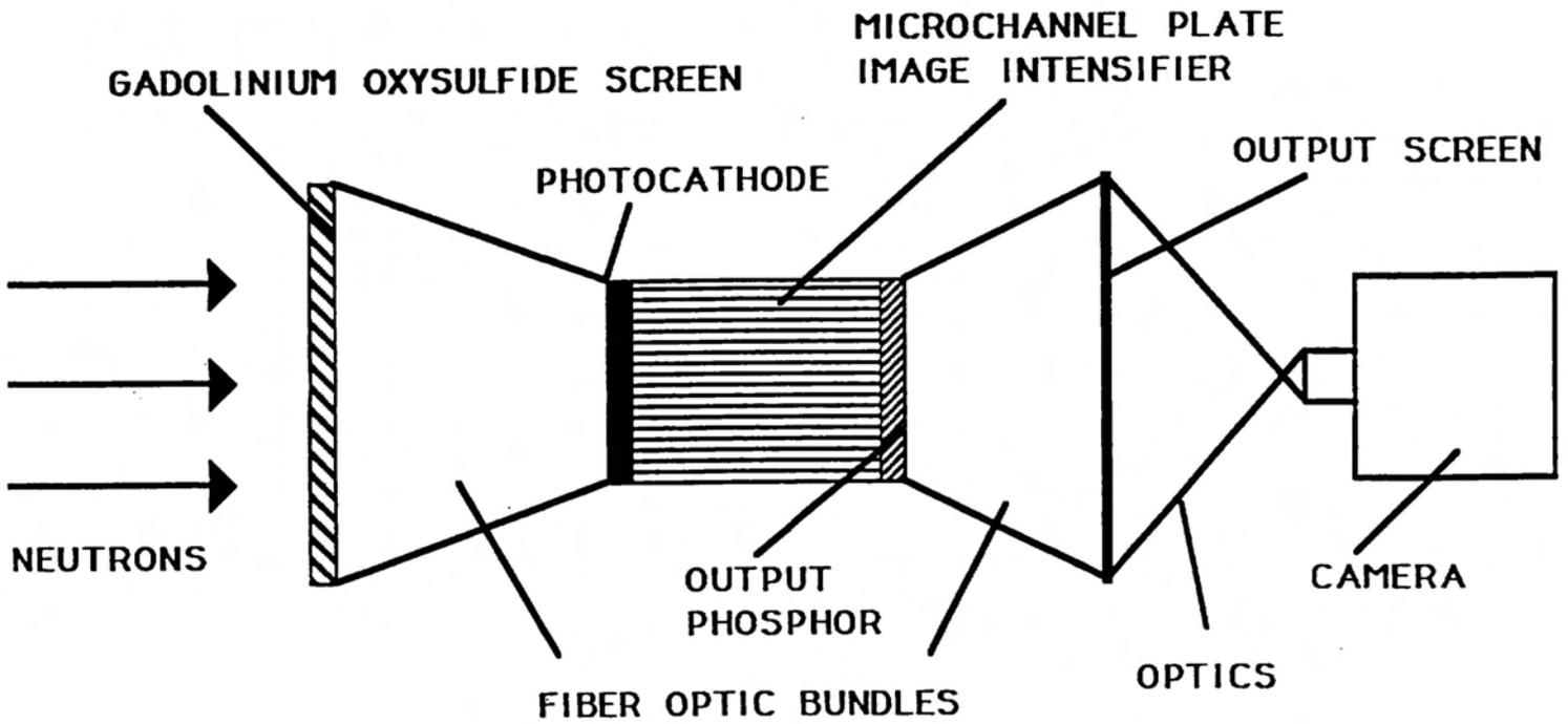
Figure 10. Representation of the LIXI NID neutron radioscopes imaging system.
