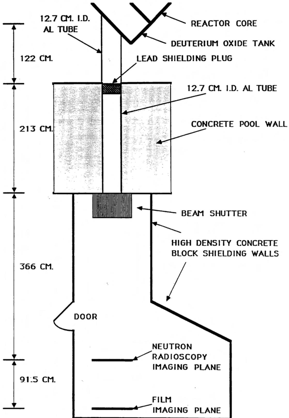
Figure 3. Spatial relationships of the horizontal neutron radiography port.
