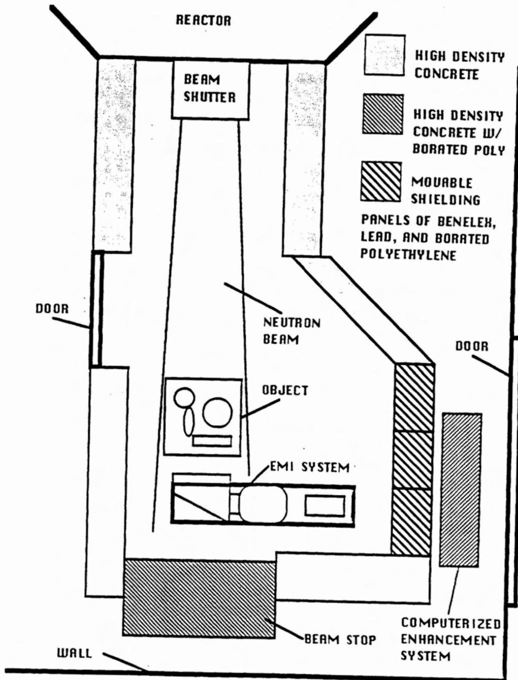
Figure 4. Construction materials used in the horizontal neutron radiography port.
