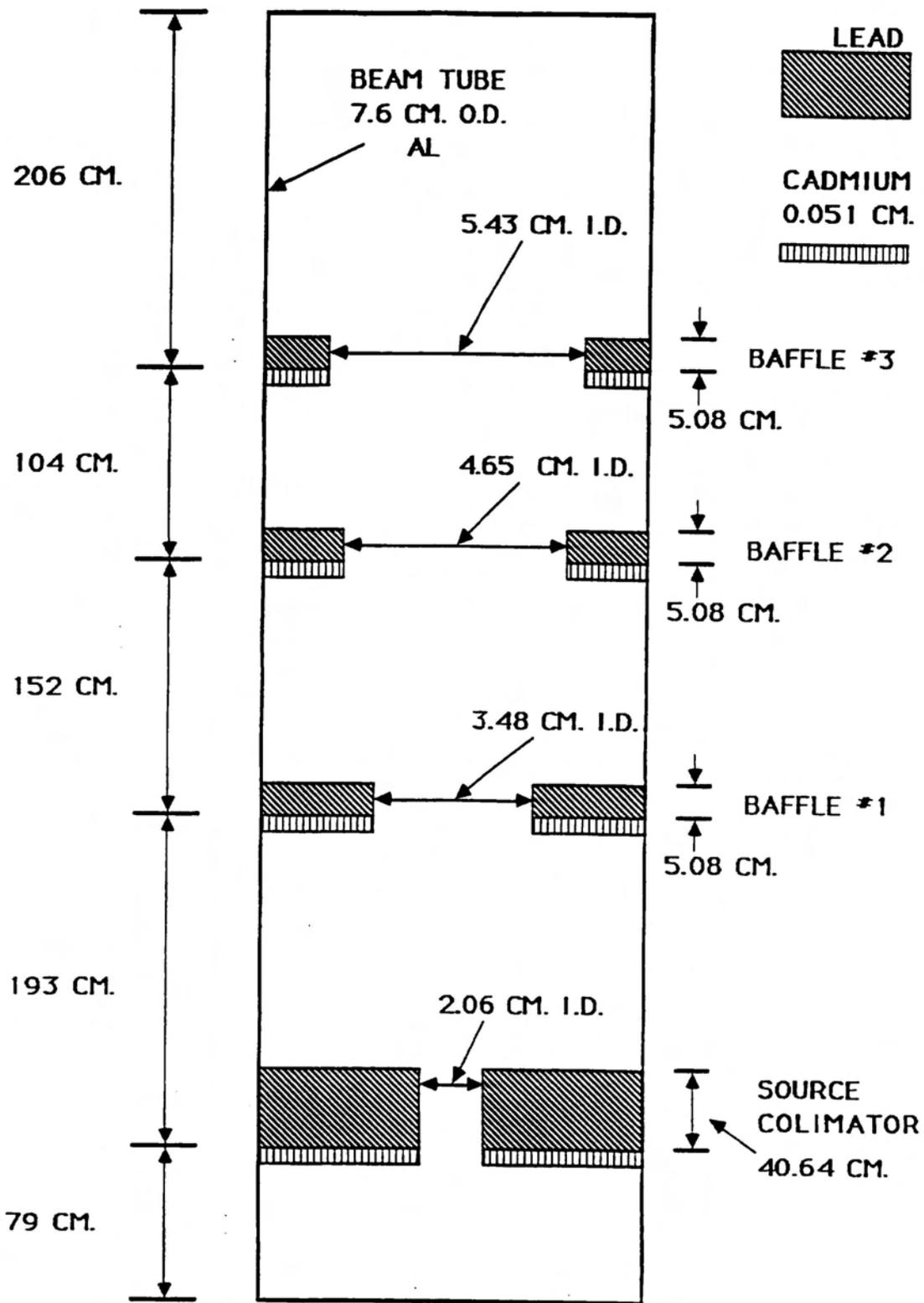
Figure 6. Details of the internal structure of the vertical beam tube.
