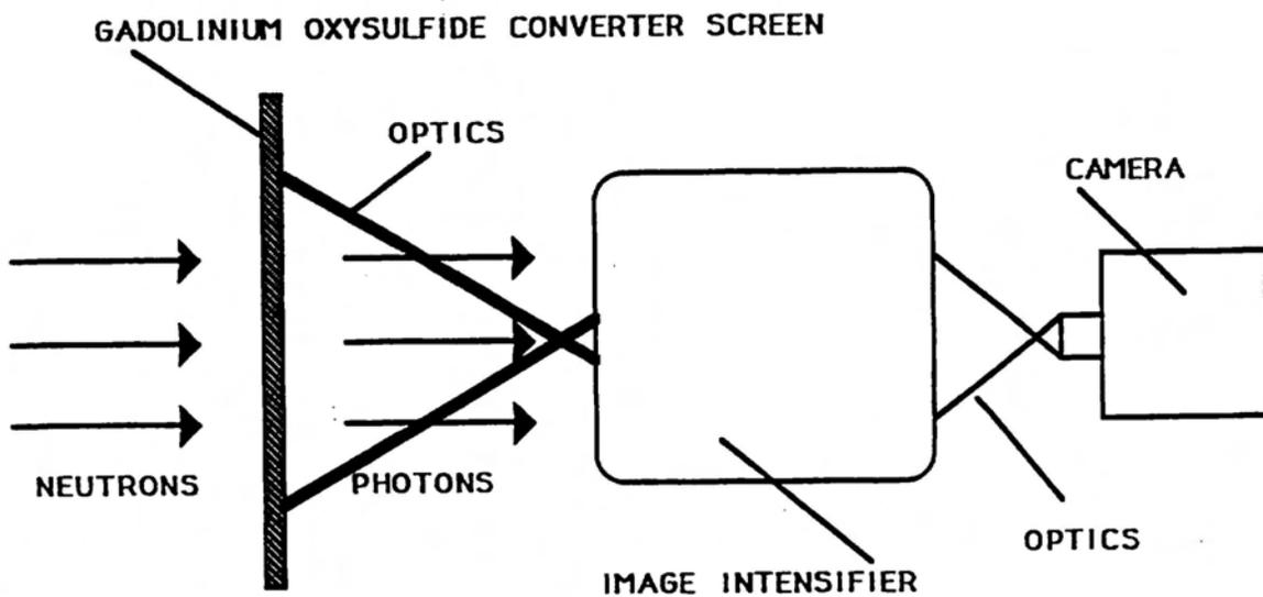
Figure 9. Example of the first generation neutron radiography imaging systems.
